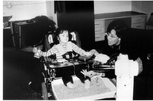
Fig. 9. The robot arm provides a means for the child to engage in a play activity by digging up an object and handing it to her adult play partner.
