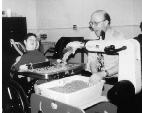
Fig. 1. The robotic system. The robot arm is shown in the foreground. The child was able to dig and find objects hidden in a tub of dry macaroni.
