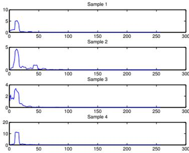
(a) PSD of four randomly chosen samples from the Assault Amphibian Vehicle (AAV) set.
