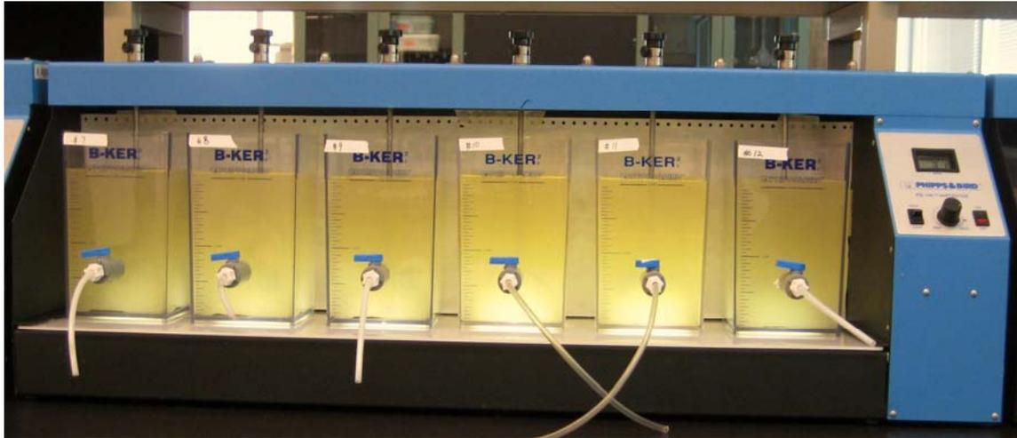
Figure 2: Jar-Test Apparatus: Phipps & Bird PB-700™ JarTester
