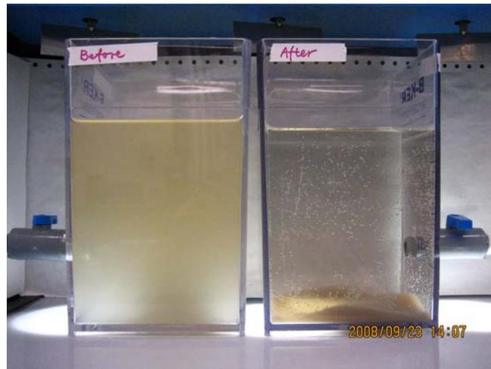
Figure 18: Comparison of the OSPW before and after coagulation-flocculation and sedimentation processes using 250 mg/L alum and 5 mg/L CTI TL in the optimum jar-test conditions
