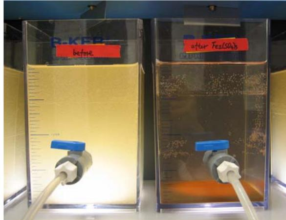
Figure 36: OSPW before and after coagulation-flocculation and sedimentation processes using 250 mg/L ferric sulfate and 1 mg/L CTI TL
