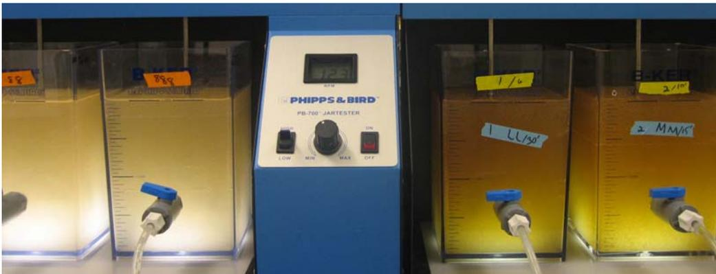
Figure 41: Comparison of the coagulation-flocculation processes process using alum and ferric sulfate as a coagulant (left: 250 mg/L alum + 5 mg/L CTI TL; right: 250 mg/L ferric sulfate + 1 mg/L CTI TL)
