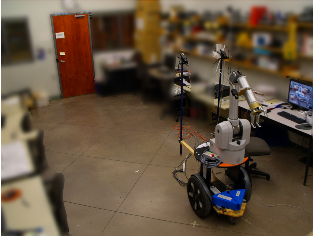
Figure 5.20: The teleoperated mobile manipulator in the initial setting to open a door.
