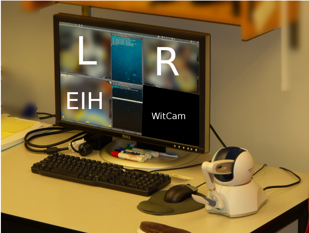
Figure 5.1: The Teleoperation station showing the Phantom Omni (on the right), a keyboard and the monitor. The monitor displays (left to right and top to bottom) the left and right overview cameras, the eye in hand camera, and the bird’s eye documenting camera. This minimal setting is used to teleoperate the full robot.
