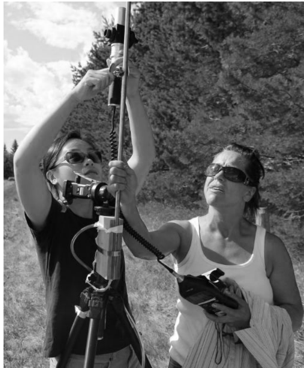
Figure 2.5: Attaching a Casella dust monitor to a tripod at the height of 2 m in the field.
