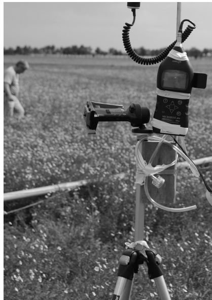
Figure 2.4: A casella dust monitor was attached to a tripod at the height of 2 m in the field.
