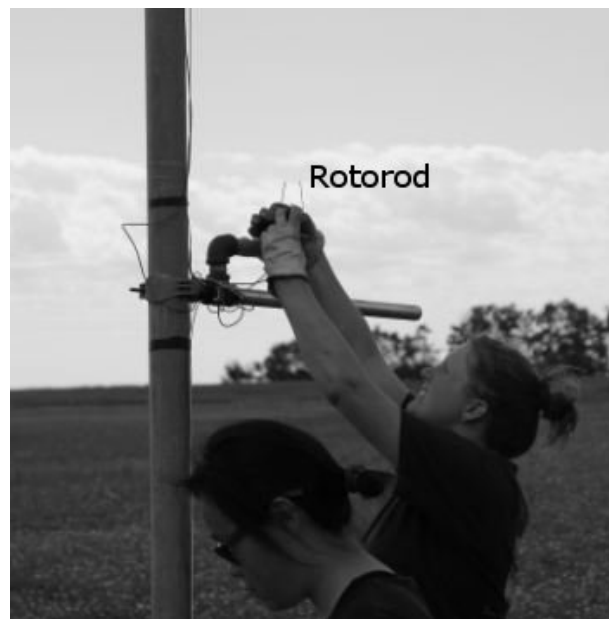
Figure 2.8: Placing a Rotorod onto a stand at the height of 2 m
