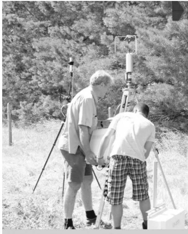
Figure 2.10: Attaching a data logger onto a sonic anemometer.
