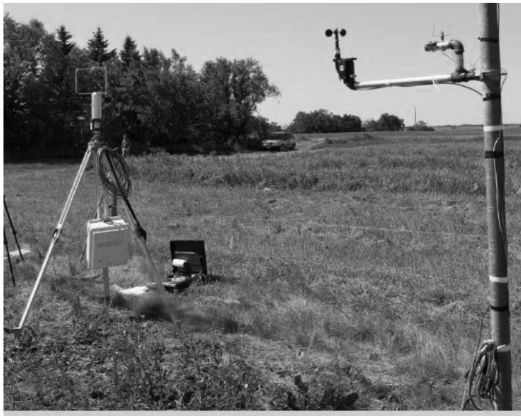
Figure 2.9: A sonic anemometer, a cup anemometer and a Rotorod on a stand of 2 m high in the field.
