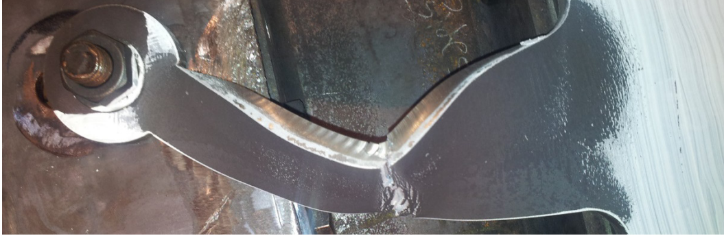
Figure 5-42: Test Specimen #5 - Shear Link Damage
