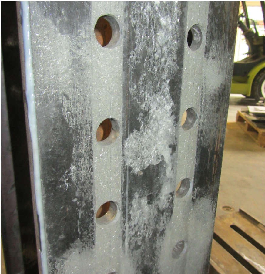
Figure 6-3: Post-Experiment Surface Condition of Non-asbestos Glass Fiber Reinforced Friction Sheet Material
