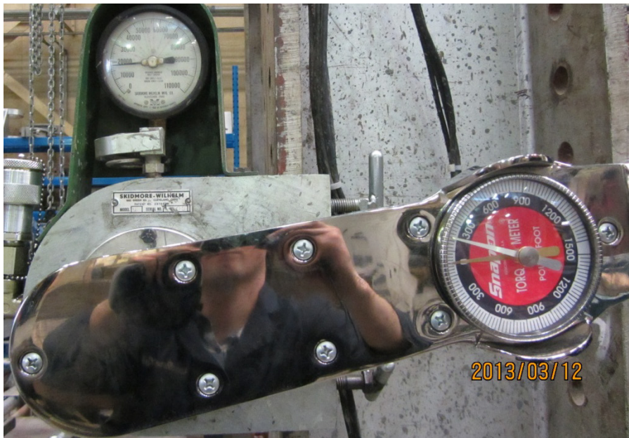
Figure 4-4: Bolt Pretension Test (Torque Wrench Calibration)
