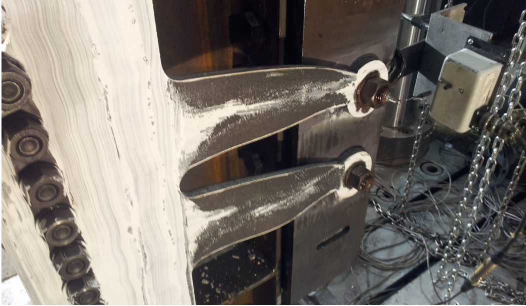
Figure 5-10: Test Specimen # 1 – Buckling of Steel Fuse Plate – Cycles 9 and 10
