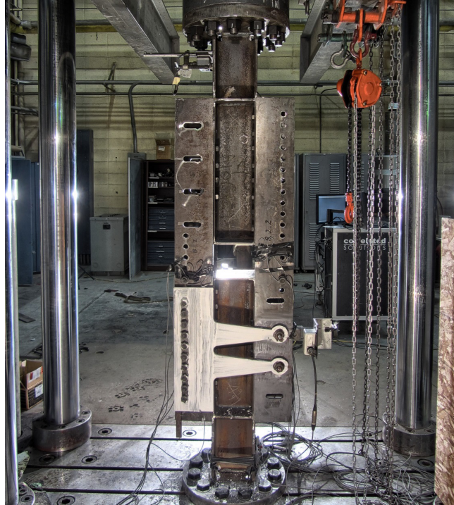
Figure 5-5: Test Specimen # 1 - Prior to Test
