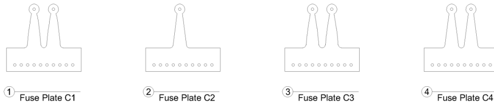
Figure 4-12: Ductile Steel Fuse Plates - Schematic Diagram
