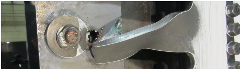
Figure 5-23: Test Specimen 3 - Shear Link Fracture
