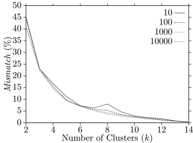
Figure 4.1: Clustering error for varied iterations of  $\epsilon$ -greedy spectral clustering when using similarity matrix  $S$  from `gcc`
