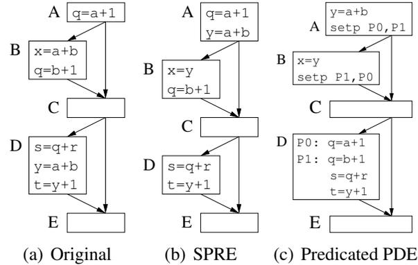
Figure A.3: Speculative PRE and PDE using predication
