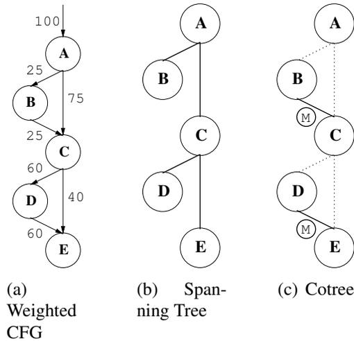
Figure B.3: Finding the minimum instrumentation required for edge profiling
