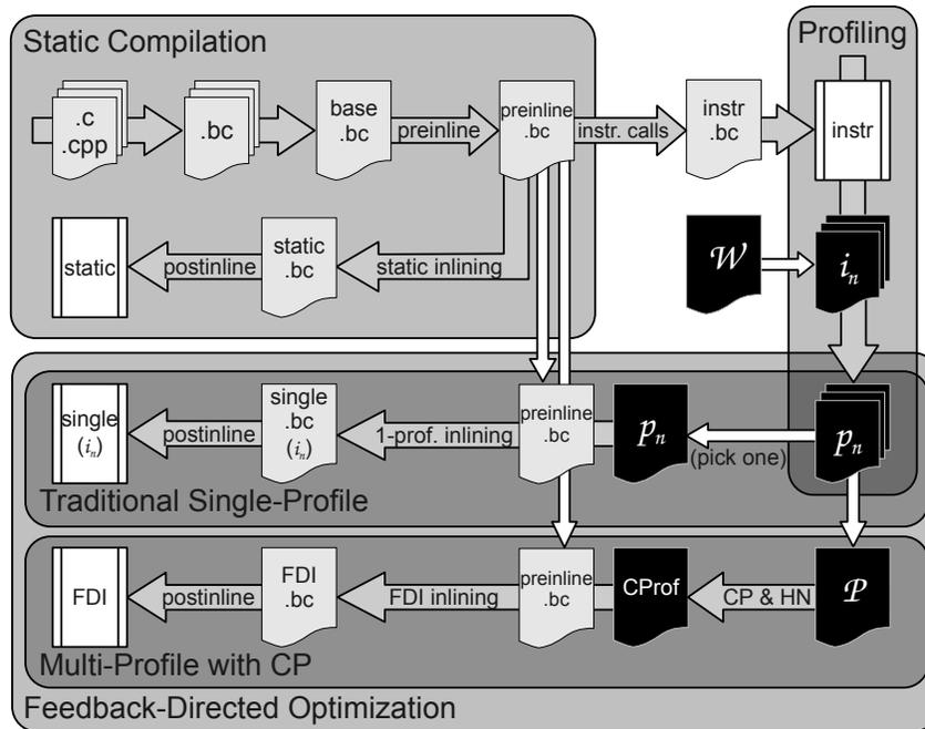
Figure 7.1: Overview of FDO program compilation with LLVM for static and FDI inlining. Postinline .bc files are omitted for simplicity.
