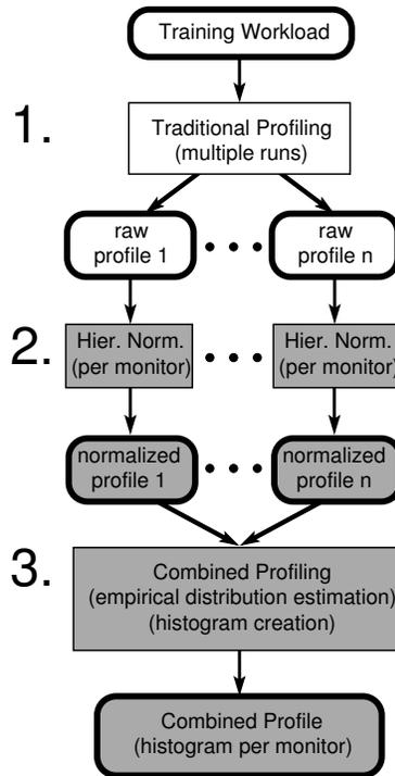
Figure 5.1: Three phases of combined profiling: 1) profile each input, 2) normalize each profile, and 3) combine the profiles into a distribution model.
