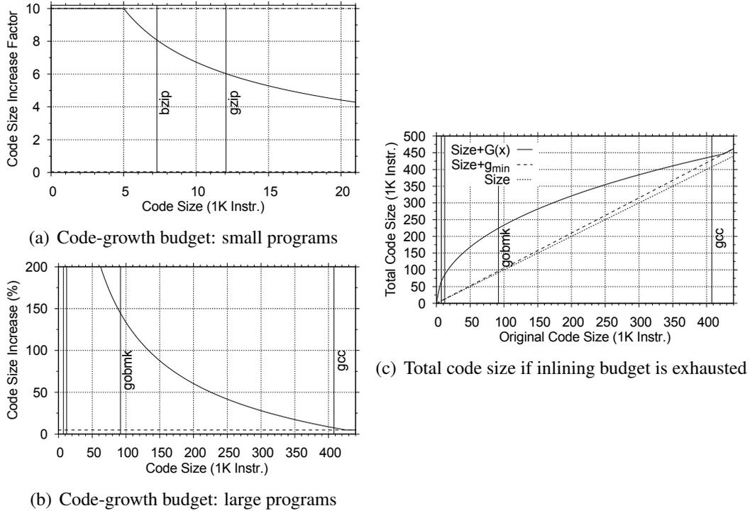
Figure 6.2: Allowable code-growth budget for FDI inlining in terms of LLVM IR instructions. The initial size of `bzip2`, `gzip`, `gobmk`, and `gcc` are indicated with vertical lines.
