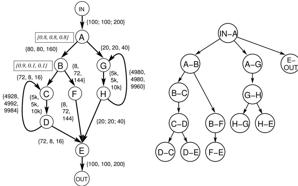
(a) A control flow graph. Edges are labeled with the raw frequencies for {P1, P2, P3}. The probabilities that the left branch is taken from nodes *A* and *B* are listed in the adjacent boxes. (b) The edge-dominator tree for Figure 5.4(a).
