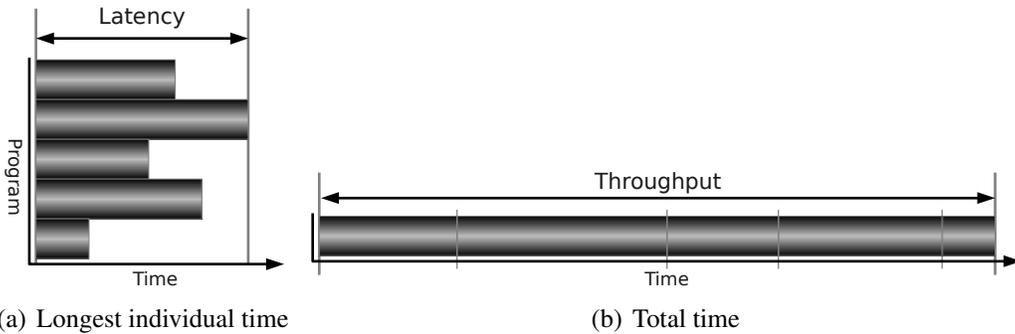
Figure 1.1: Measurements for workload evaluation using latency or throughput
