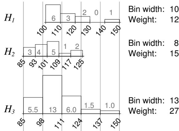
Figure 5.3: Combining histograms:  $H_1 + H_2 = H_3$
