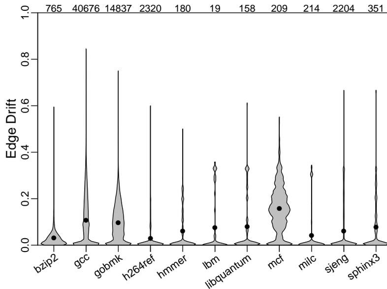
Figure 5.11: Edge-weight drift using 50-bin histograms (no points)
