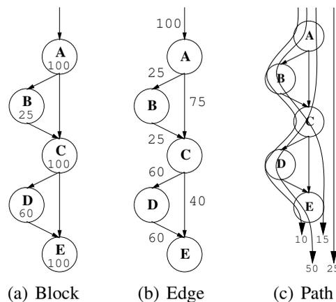
Figure B.1: Block, edge, and path profiles for a simple CFG
