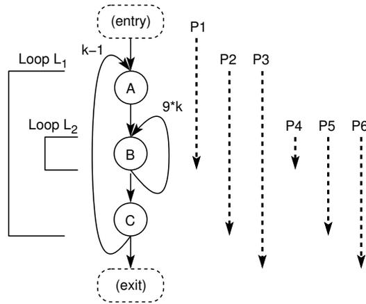
Figure 5.6: Some sub-paths through a nested loop. The outer loop  $L_1$  iterates a total of  $k$  times; the inner loop  $L_2$  iterates 10 times per iteration of  $L_1$ .
