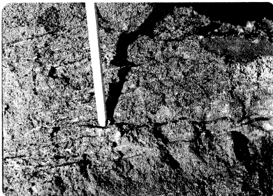
PLATE 4.3b Parting Along Cross-beds. Most of the length of the partings shown above is along cross-beds.
