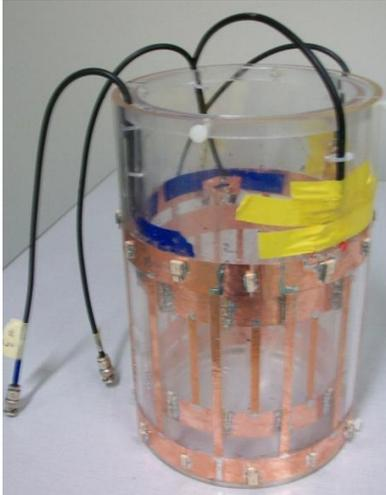
Figure 5-2: The double tuned coil used to acquire the images in Figures 5-3a and 5-4.
