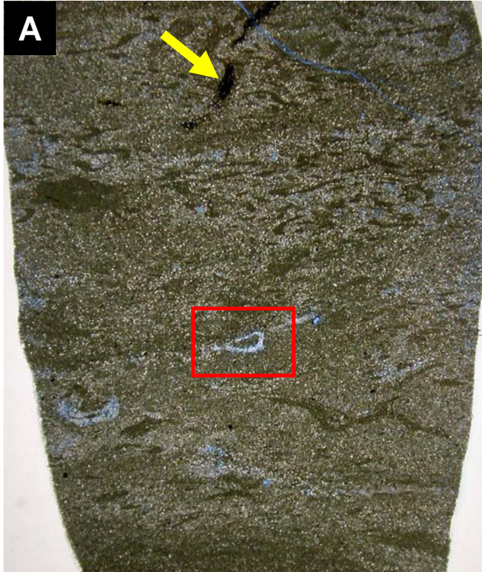
Figure 2.5 (A) Overview scan of an intensely burrowed silty shale from the Cretaceous-aged Colorado Group silts and shales (FOV is approximately 2.5 cm wide). (B) Close up of the burrow highlighted by the red box in Photo A (scale bar is 0.2 mm). The burrows in this example all have excellent preserved secondary porosity after carbonate cement dissolution. Note pyrite filled burrow (arrow) indicating these rocks were deposited in a reducing environment.
