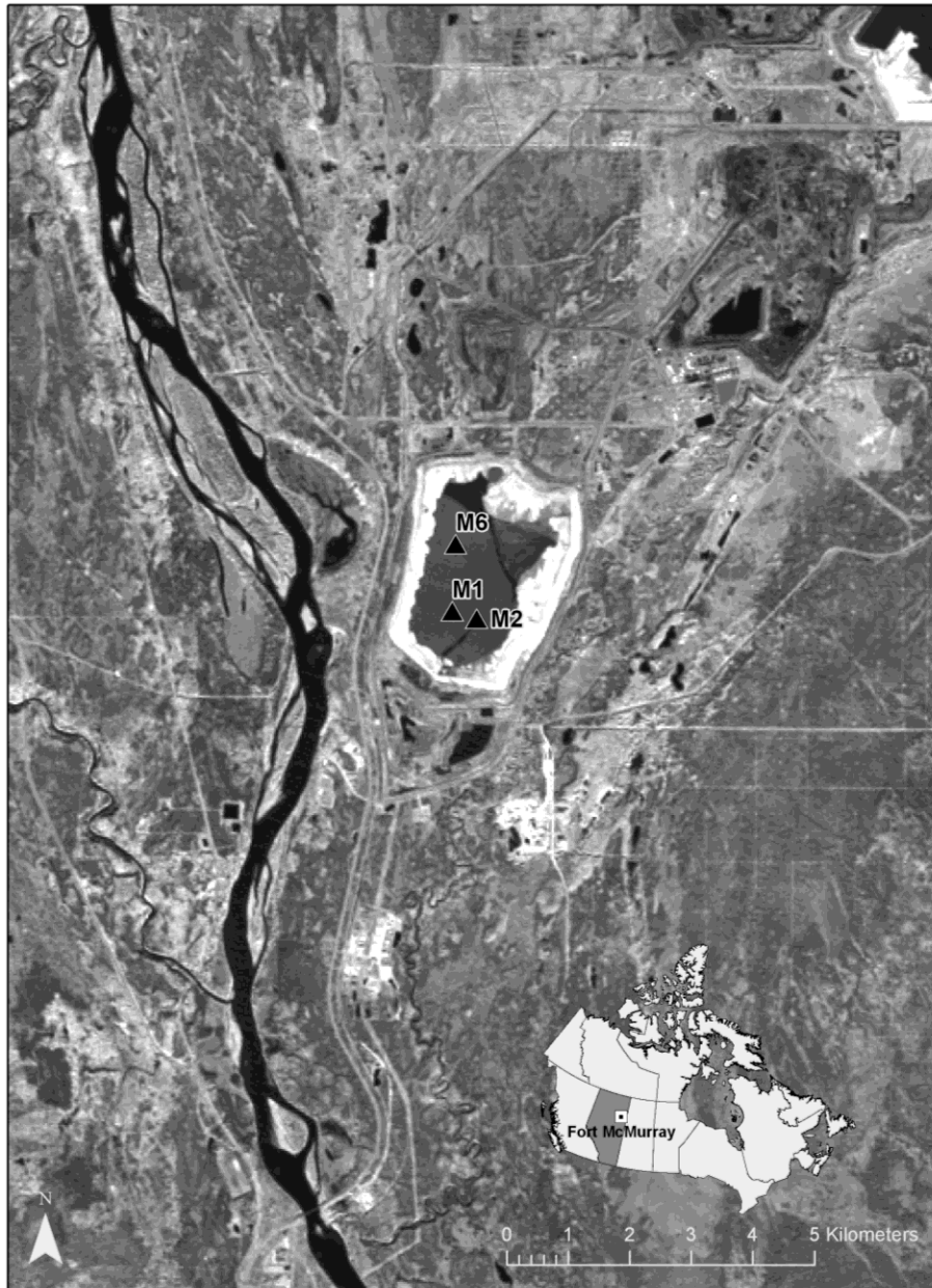
Figure 2.1. Sample locations within the tailings pond of Shell Albian Sands for M1, M2, and M6 MFT samples. Locations are marked with triangles. M4 and M5 MFT samples have been omitted because their exact sample location is unclear. The background is a false natural color composite of Landsat 5 Thematic Mapper satellite imagery of Path 42 Row 24, taken on September 14, 2009. Map was obtained from and sample locations were marked by Charlene Nielsen, Geographic Information Systems in Biological Sciences, University of Alberta.
