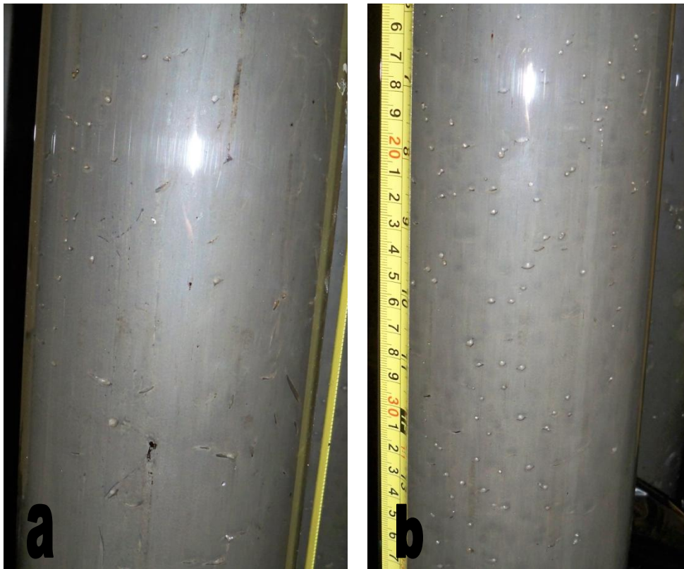
Figure B-1. Photos of duplicate settling column tailings amended with citrate: a) thin cracks are dispersed throughout tailings in one and b) many small spherical bubbles are seen dispersed throughout tailings in the other.
