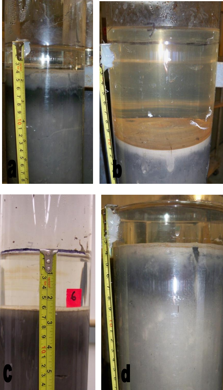
Figure 3.22. Water caps in 7-L settling column MFT: a) clear water released from baseline control MFT with few small gas bubbles in solids material; b) the slightly turbid water cap on the surface of solids material of MFT amended with citrate plus diluent plus polyacrylamide; c) clear water released from MFT amended with diluent; d) clear water released from MFT amended with polyacrylamide. Note the absence of gas bubbles in MFT of settling columns pictured in 3.22c and 3.22d.
