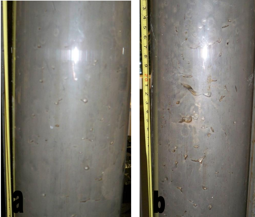
Figure B-2. Photos of duplicate settling column tailings amended with citrate plus polyacrylamide: a) small but numerous bubbles are dispersed throughout the tailings in one column and b) large gas pockets and some thin cracks are observed in the tailings of the other column.
