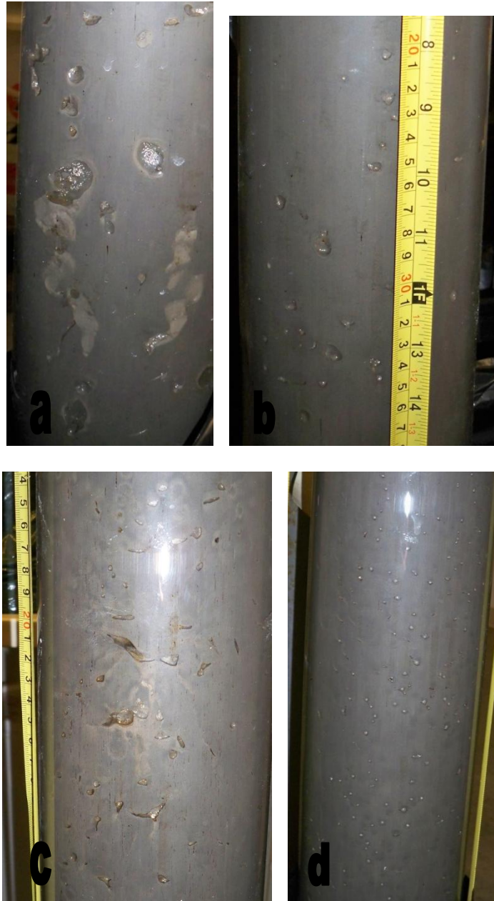
Figure 3.21. Gas bubbles in 7-L settling column MFT: a) very large gas pockets dispersed through the solids material of MFT amended with citrate plus diluent plus polyacrylamide; b) some small and mid-sized gas bubbles dispersed through the solids material of MFT amended with citrate plus diluent; c) mid-sized gas pockets formed through solids material of MFT amended with citrate plus polyacrylamide; d) numerous small gas bubbles dispersed in MFT amended with citrate.
