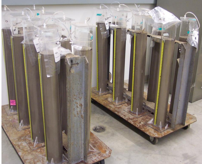
Figure 2.4. Settling columns filled with 7 L of Albion MFT, amended with citrate, diluent, polyacrylamide, or a combination of two or three of these, or with cap water (baseline control), sealed and fitted with 1 L Tedlar bags and tape measures for monitoring gas production and MFT densification.
