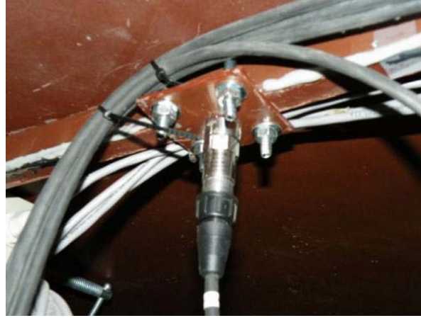
Figure 5.2. Installation of the PCB accelerometer (Terrell 2011)
