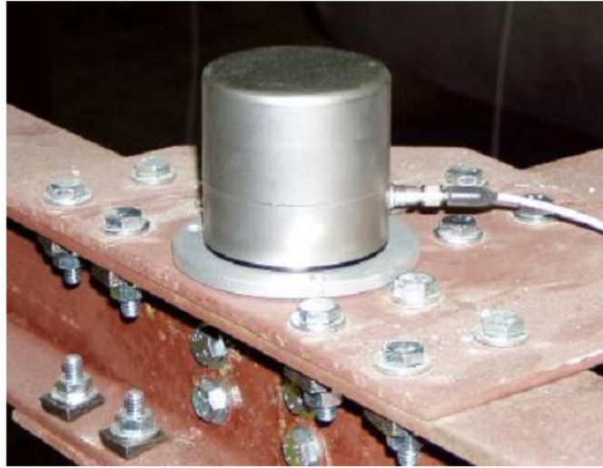
Figure 4.4. Installation of accelerometer on the structure (Gül 2009)
