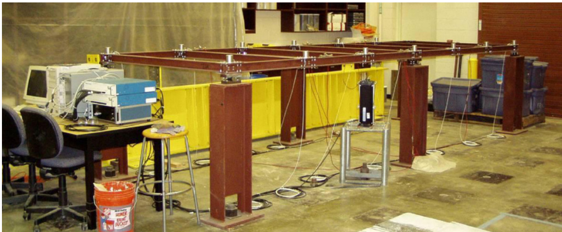
Figure 4.1. Steel grid model used for experiments (Gül and Catbas 2011)
