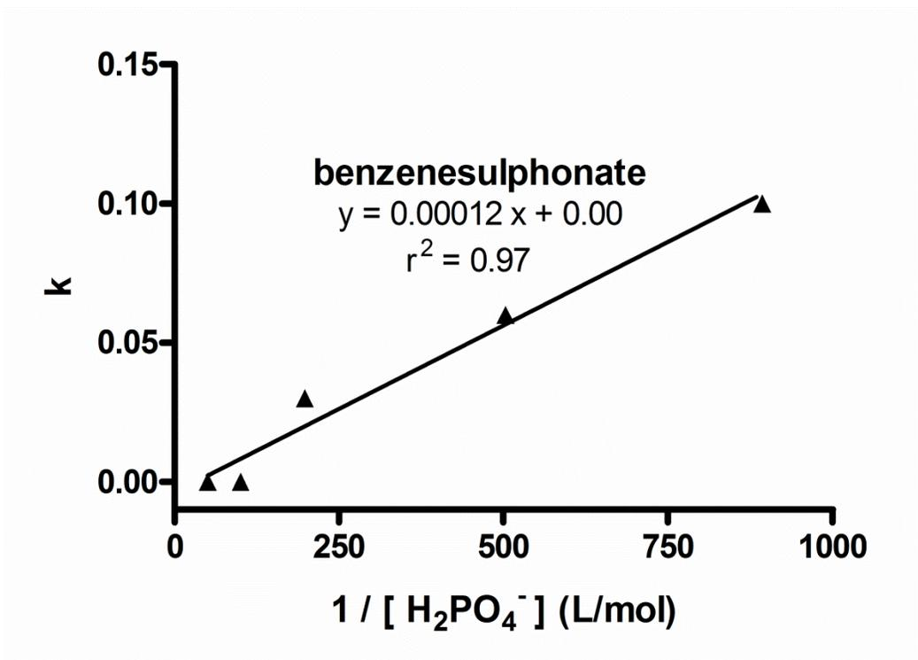
**Figure 3-9.** Retention of benzenesulphonate on HC-T after 500 column volumes of acid treatment. Conditions as in Figure 3-6. Error bars are smaller than the graph marks.
