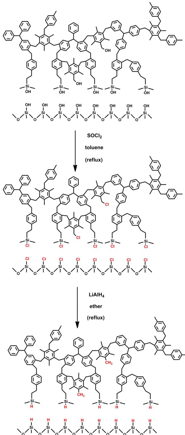
**Figure 4-4.** HC-T modification to remove residual polar groups
