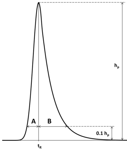
**Figure 1-3.** Graphical determination of the asymmetry factor ( $B/A$ ) for a tailing peak
