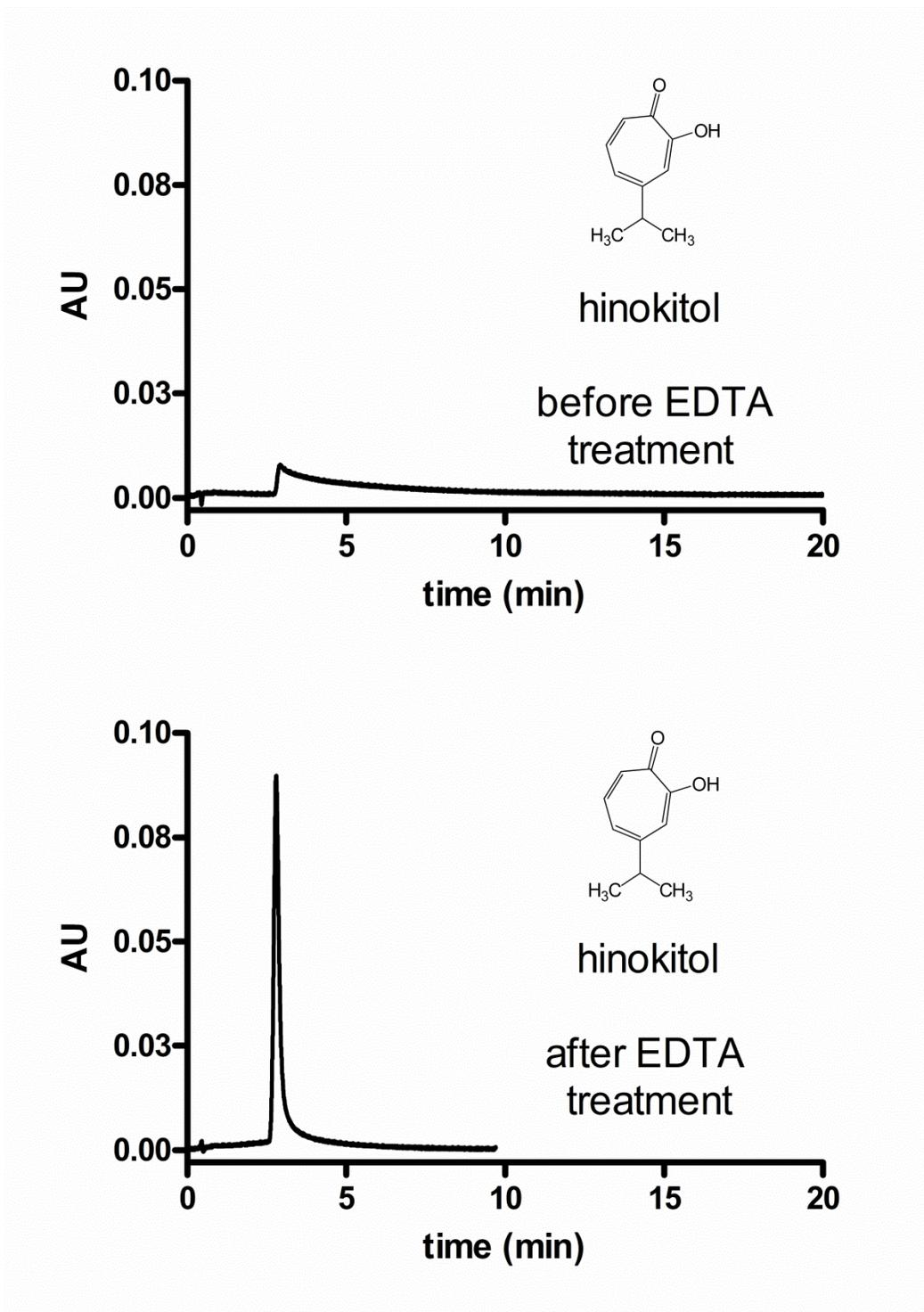
**Figure 3-12.** Effect of the EDTA treatment on the chelating properties of the HC-T column. Conditions as in Figure 3-2c.
