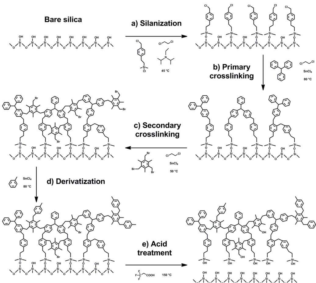
**Figure 2-4.** Synthesis of toluene derivatized hypercrosslinked silica-based stationary phase (adapted from [25]).
