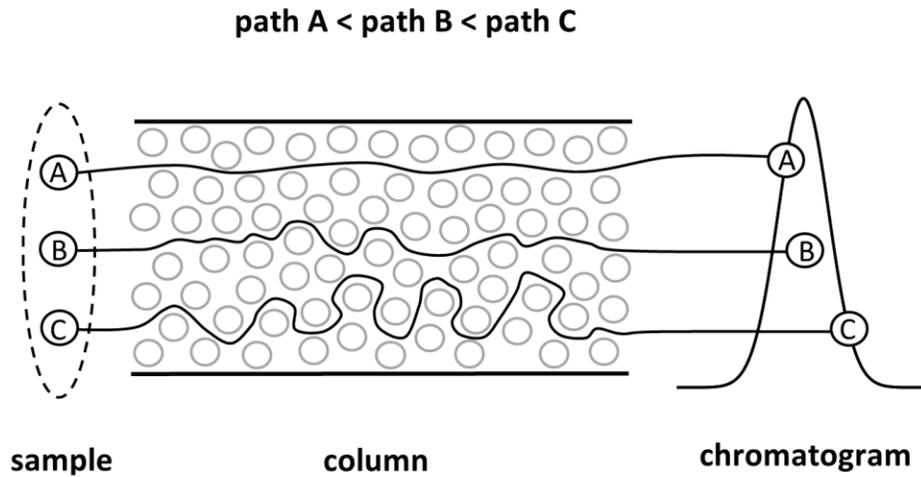
**Figure 1-4.** Schematic representation of multiple path band broadening
