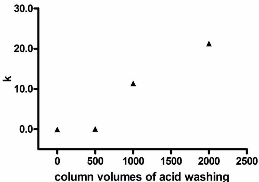
**Figure 3-5.** Retention of benzenesulphonate as a function of the HC-T column acid treatment. Conditions as in Figure 3-2. Error bars are smaller than the graph marks.
