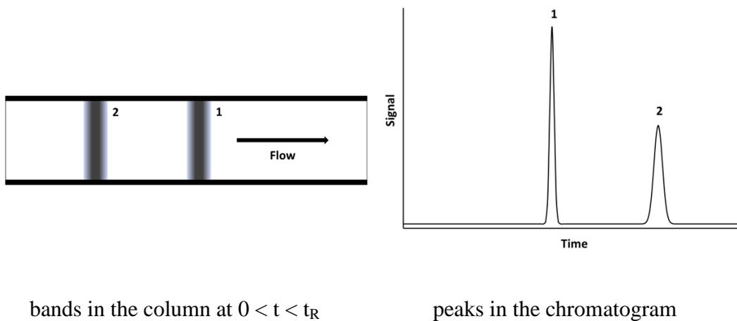
**Figure 1-1.** Column separation and the resultant chromatogram
