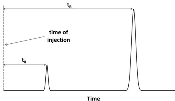
**Figure 1-2.** Illustration of retention time ( $t_R$ ) and dead time ( $t_0$ )
