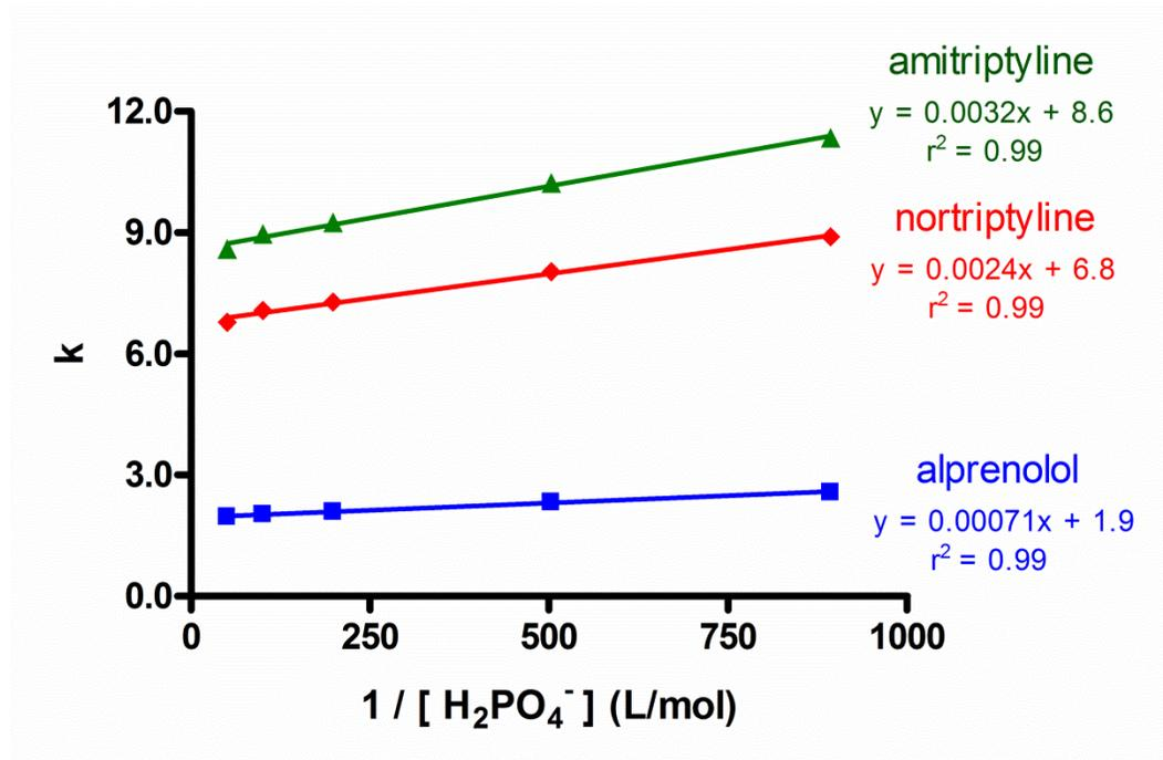
**Figure 3-6.** Retention of the basic drugs on HC-T before acid treatment. Conditions: 30 % ACN/water, phosphate buffer pH 3.0; injection volume 0.5  $\mu$ L; amount injected 0.025 nmol; temp. 40  $^{\circ}$ C; detection at 254 nm. Error bars are smaller than the graph marks.
