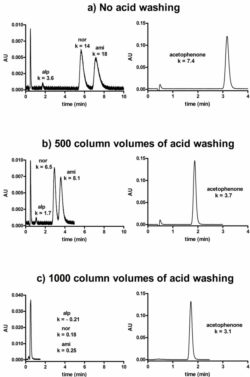
**Figure 3-2.** Effect of the acid washing on the retention of basic and neutral compounds on the HC-T column. Conditions: isocratic elution, 29 % acetonitrile in water, buffered with 0.1% formic acid, pH 3.0; 1.0 ml/min; 40 °C, 0.025 nmol amount of each basic drug and 0.2 nmol of acetophenone; 0.5  $\mu$ L injection; detection at 254 nm. The HC-T column was acid treated as detailed in Section 3.2.4.
