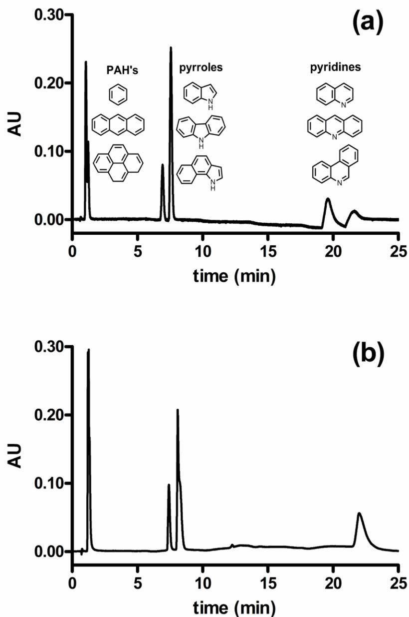
**Figure 3-4.** Group-type separation of nitrogen aromatic heterocycles on (a) HC-T synthesized herein and (b) HC-T in reference [7]. Conditions: 5.0 x 0.46 ID mm HC-T column subjected to 500 column volumes of acid washing; elution, 20 min step gradient starting at 5% dichloromethane (DCM) in pure hexane and increasing by 20% DCM every 4 min; 1 ml/min; 40 °C; detection at 254 nm.
