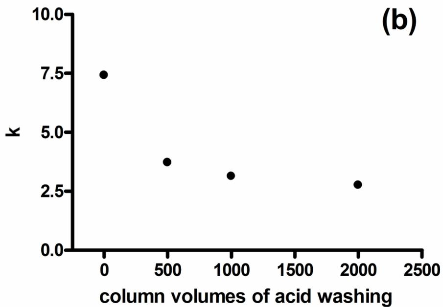
**Figure 3-3.** Retention of basic (a) and neutral analytes (b) on HC-T as a function of the acid washing. Conditions as in Figure 3-2. Error bars are smaller than the graph marks.
