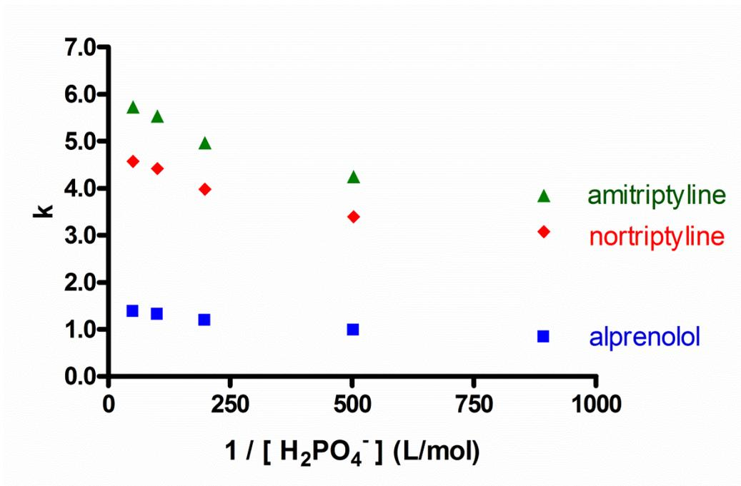
**Figure 3-8.** Retention of basic drugs on HC-T after 500 column volumes of acid treatment. Conditions as in Figure 3-6, except that the column has been conditioned as described in Section 3.2.4. Error bars are smaller than the graph marks.
