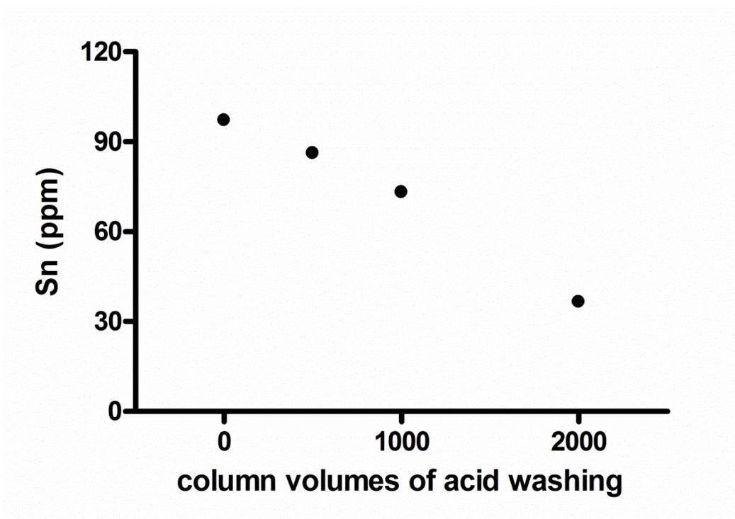
**Figure 2-5.** Tin content in the stationary phase as a function of the number of acid wash cycles of HC-T *batch I*. No replicates were run.
