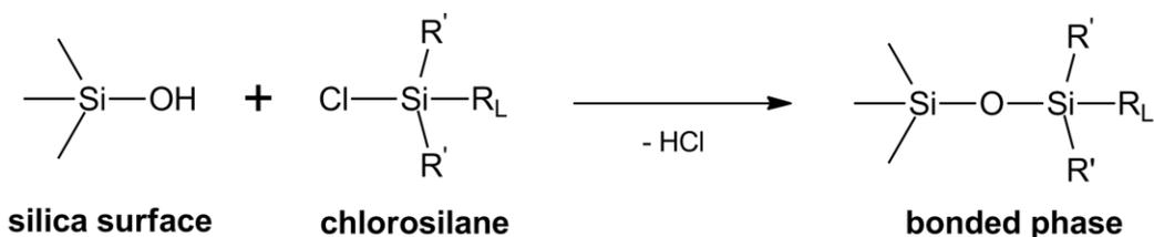
**Figure 1-7.** Silanization of silica producing a bonded stationary phase
