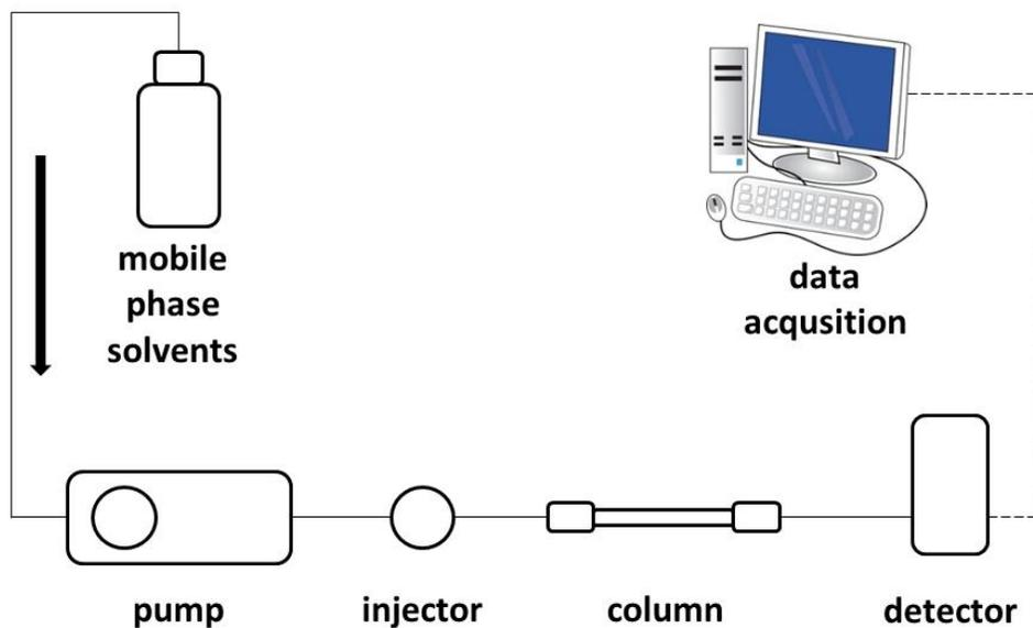
**Figure 1-5.** Basic elements of an HPLC system
