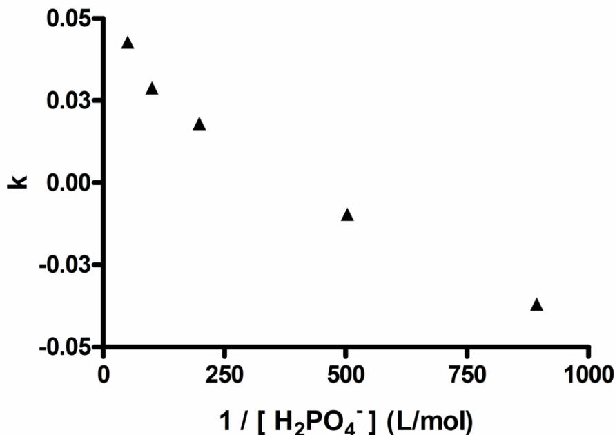
**Figure 3-7.** Retention of benzenesulphonate on HC-T before acid treatment. Conditions: 30 % ACN/water, phosphate buffer pH 3.0; injection volume 0.5  $\mu\text{L}$ ; amount injected 0.025 nmol; column temperature, 40  $^\circ\text{C}$ ; detection at 214 nm. Error bars are smaller than the graph marks.
