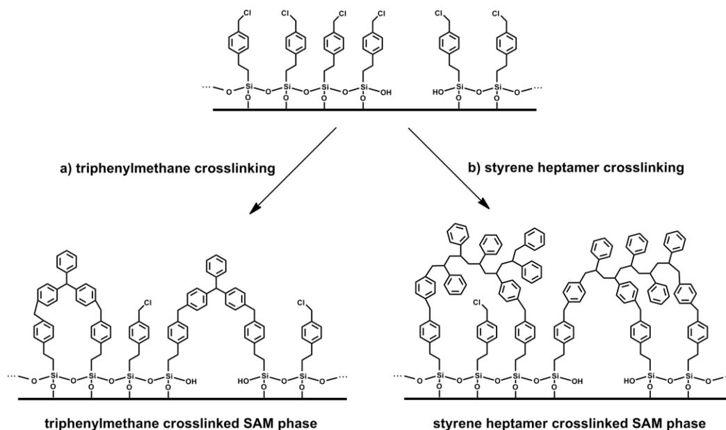
**Figure 2-2.** Crosslinking of self-assembled monolayer stationary phases
