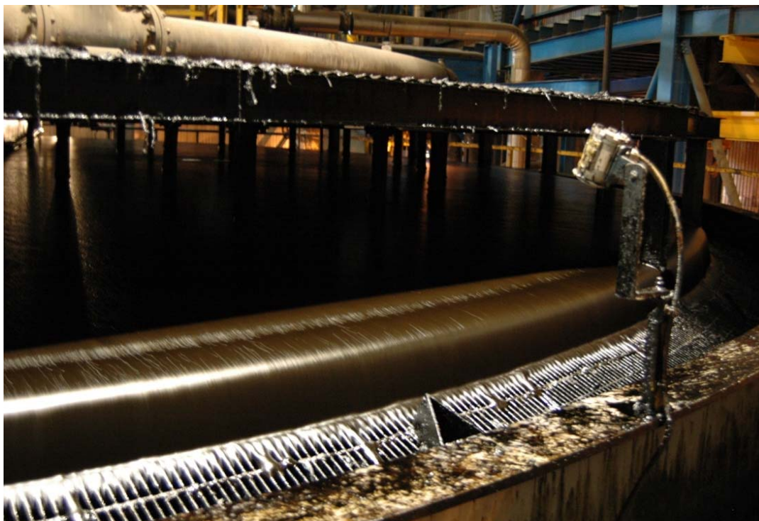
Figure 5.2: Top view of the industrial separation cell at Suncor Energy Inc. The lighter bitumen froth overflows from the top of the separation cell and transported for further processing.
