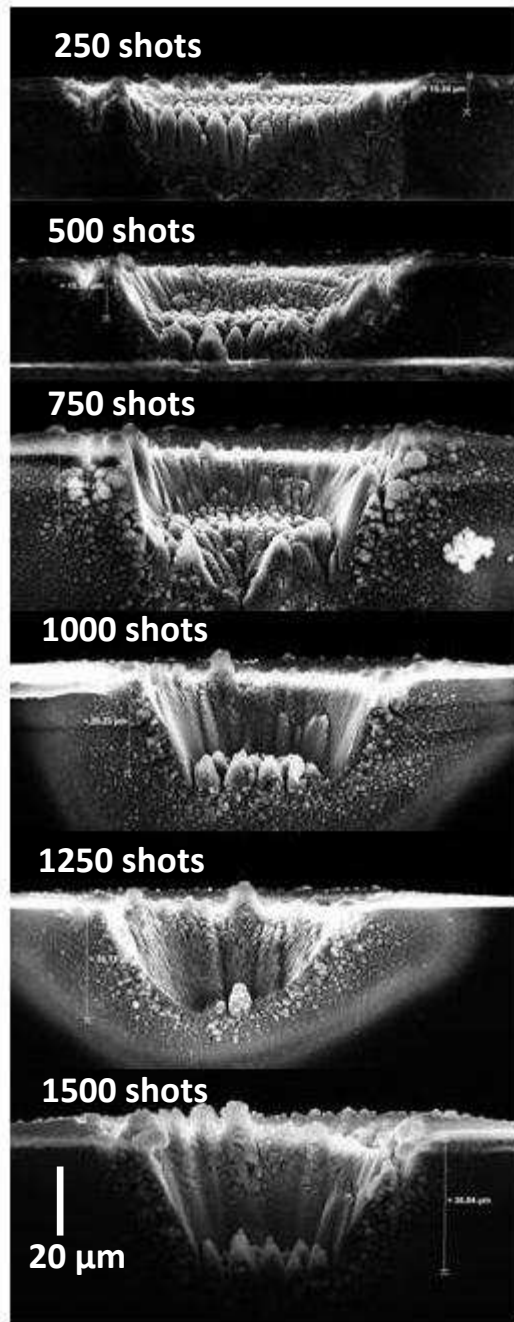
Figure 7.11: Cross sectional view of the ablation hole for different shot accumulations at a fluence of 1.4 \text{ J/cm}^2
