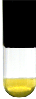
Figure 4.10: Formation of Yellowish Phase at the Same Salinities as in Guideline Jars, 1 wt% NaCl Concentration, C_{16} - Diluted Bitumen (4 : 1 wt ratio), [AOT]_{Overall} = 2.5 \text{ wt}\%
