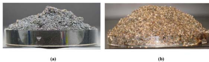
Figure 4.14: Color Change in Contaminated Soil (a) before Washing (b) after Washing
