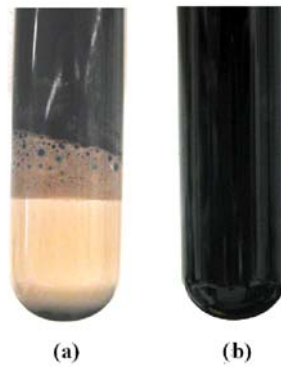
Figure 4.9: (a) Formation of Brownish Phase at 0.1 wt% Brine Solution, C_7 -Diluted Bitumen (4 : 1 wt ratio), [AOT]_{Overall} = 2.5 \text{ wt}\% - (b) No Distinguishable Interface at the Same Salinity, C_{16} -Diluted Bitumen (4 : 1 wt ratio), [AOT]_{Overall} = 2.5 \text{ wt}\%
