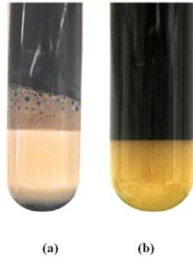
Figure 4.12: (a) Brownish Phase Caused Inhomogeneity and Formation of Gel-Like Materials in the Mixture While Quantifying Water Content at 0.1 wt% NaCl Concentration, C_7 -Diluted Bitumen (4:1 wt ratio), [AOT]_{Overall} = 2.5 \text{ wt}\% (b) the Same Mixture after Adding Acetone in Order to Homogenize the Mixture, as it is shown acetone dissolved the gel-like material and the brownish phase
