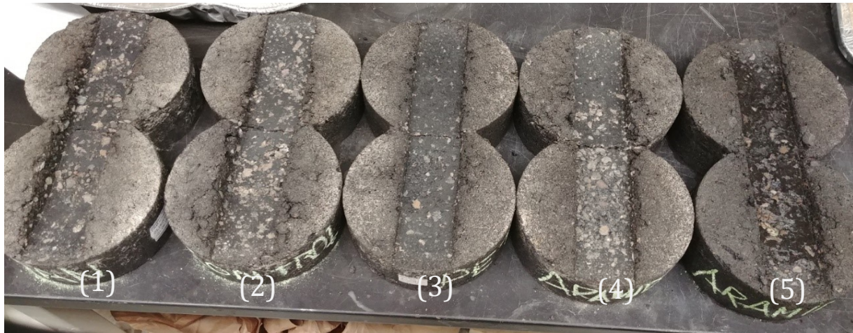
Figure 4-5: Rutting developments of: (1) PAN 0.065%; (2) CONTROL mix; (3) PET 0.1%; (4) ARAMID 0.0065%; (5) ARAMID 0.065%
