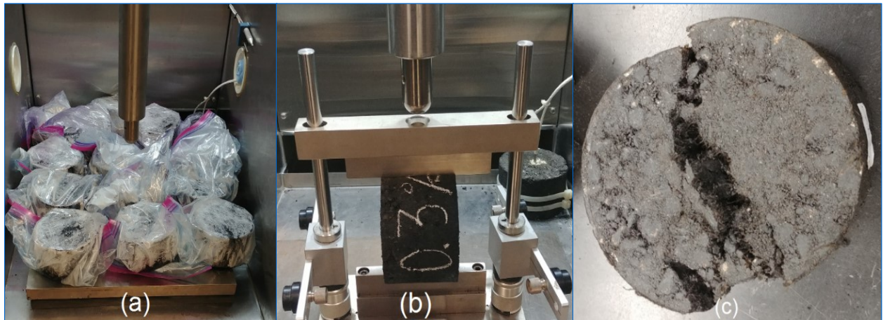
Figure 3-2: ITS test process: (a) frozen samples, (b) application of force to the sample, and (c) a broken sample
