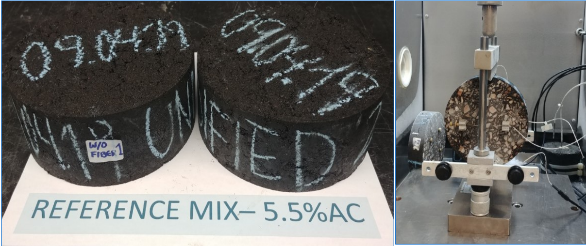
Figure 3-5: (a) IDT samples, (b) test configuration
