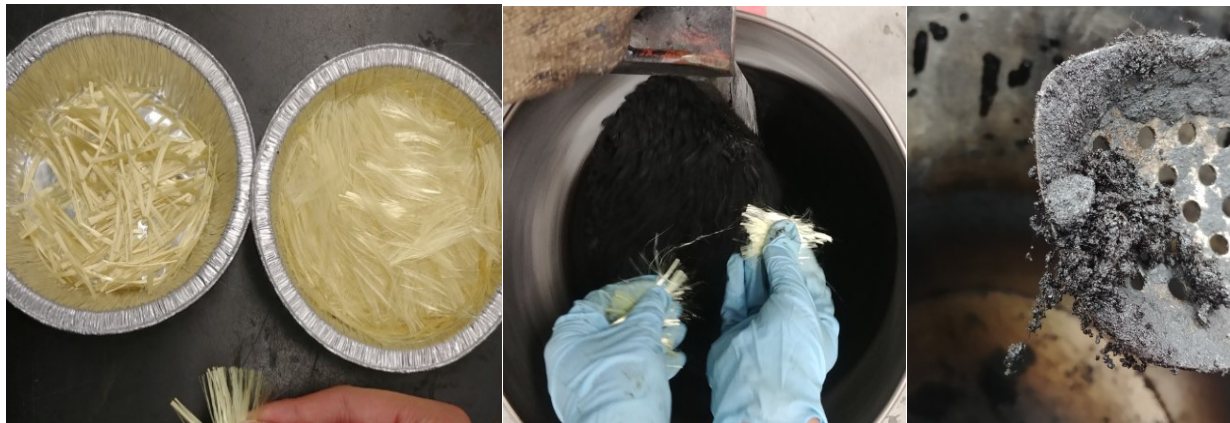
Figure 5-2: (a) Manual separation process for uncoated aramid fibers; (b) uncoated Aramid fibers being poured into the mixing bucket; (c) aggregate-binder-fiber interlock result
