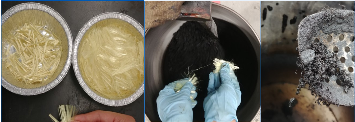
Figure 4-3: (a) Manual separation process of uncoated aramid fibers; (b) Uncoated Aramid fibers being poured into the mixing bucket; (c) aggregate-binder-fiber interlock result
