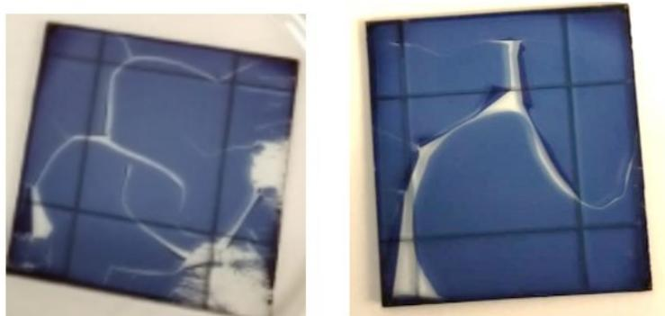
Fig. 2.12: Visual appearance of two glass/ITO/PEDOT:PSS/PM6:BTP-BO-4Cl samples (no thermal treatment) after spin-coating deposition of PFN-Br from a methanol solution.
