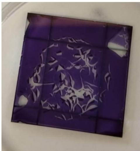
Fig. 3.22: Cracking effect of PFN-Br/MeOH on the active layer if the electron transport layer is spin coated after thermal annealing.
