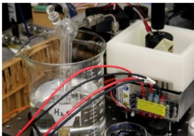
Fig. 2.14: Image of the group’s computer-controlled solvent vapor annealing system. A full schematic and detailed explanation of its components is reported by Jin et al. [23].
