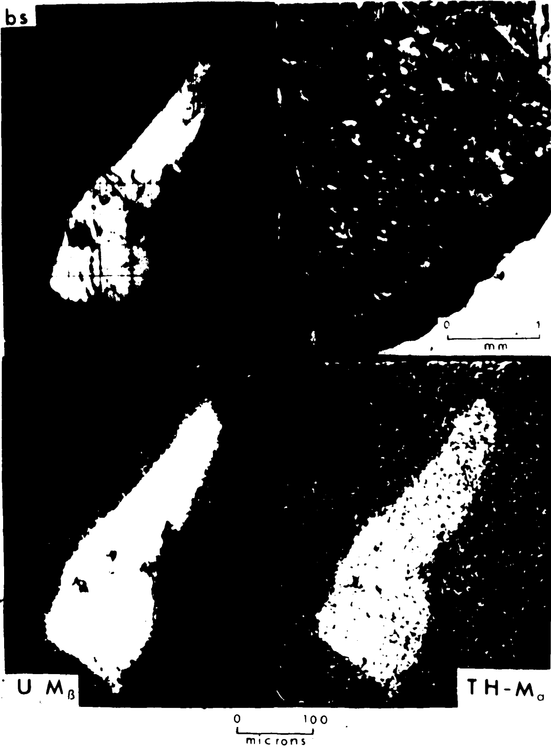
Backscatter electron and elemental photographs of uraninite 32-A. In- cluded is a phase contrast photomicrograph of the grain in biotite.
