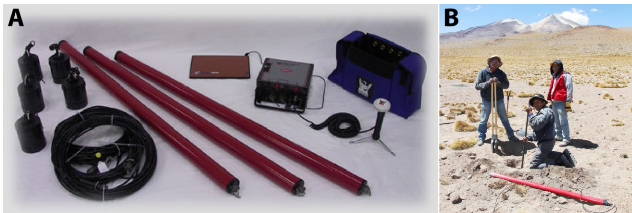
Figure 5.1: (A) Components of the Phoenix V5-2000 MT system. Shown from left to right are: porous-pot electrodes, connection cables, magnetic induction coils (for x, y, and z components), a laptop to process and store data, the MTU data acquisition unit, and a GPS antenna for time synchronization. (Photo from http://www.phoenix-geophysics.com ). (B) Installing a magnetotelluric site (1495O31-11). Photo was taken October 31, 2011, looking east towards Volcan Uturuncu.
