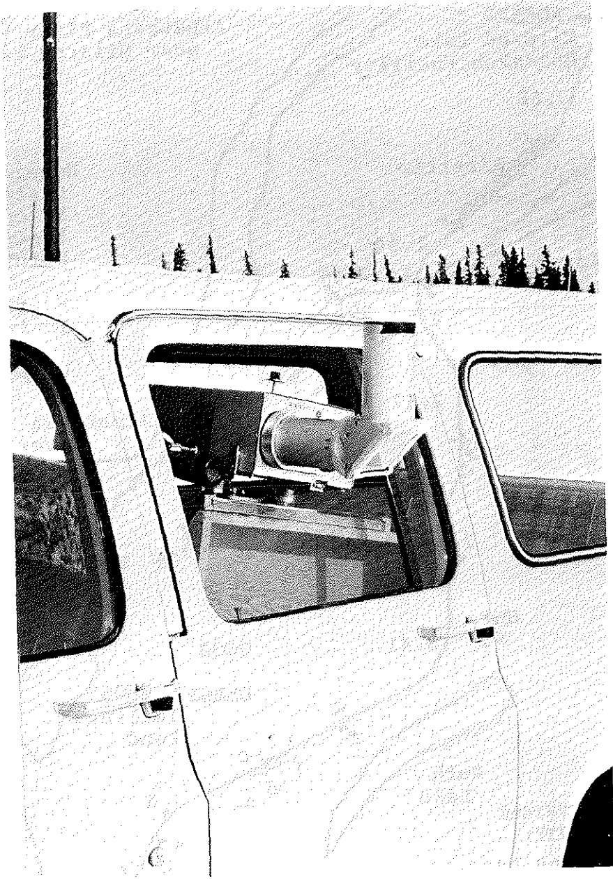
Figure 6.2. The COSPEC traversing vehicle showing the viewing telescope pointing vertically upwards.
