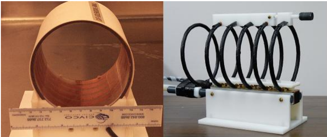
Figure 3.3 - CAT solenoid coil (left) and black solenoid coil (right). The strips of copper winding can be seen in the bore of the CAT coil, while the black coil has windings made from cylindrical copper pipe.
