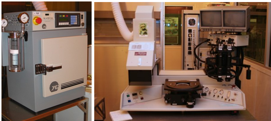
Figure 4-5 YES HDMS oven (left) and ABM mask aligner (right) at nanoFAB, University of Alberta [156].
