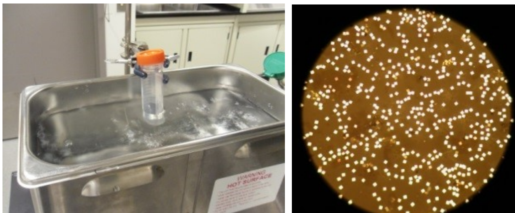
Figure 4-24 Sonication to detach devices from membrane filter into the hybridization buffer (left). Optical microscopic view of membrane filter containing 25 \mu\text{m} devices (right).
