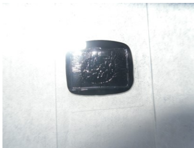
Figure 4-32 A cover slip was used to spread the oligo solution over the substrate.
