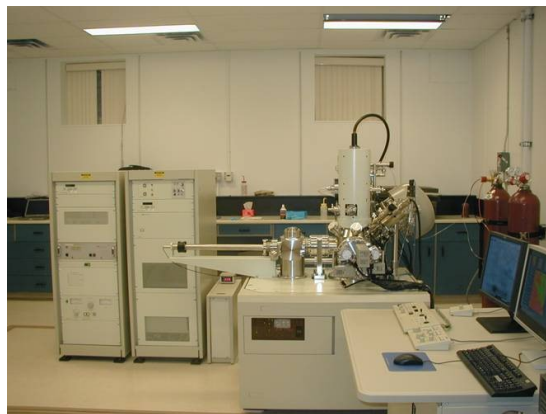
Figure 4-17 JAMP-9500F scanning electron microscope at ACSES, University of Alberta [156].
