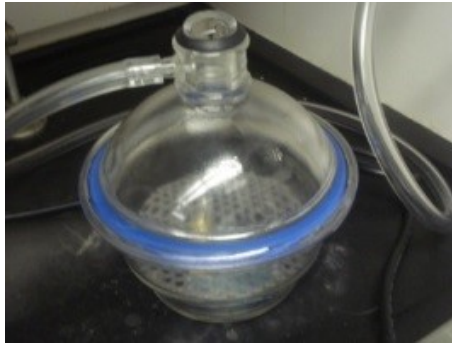
Figure 4-30 Small vacuum desiccator used to perform CVD for SAM formation on the Si substrate.
