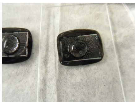
Figure 4-31 A drop of oligo solution to attach complementary DNA to the devices.
