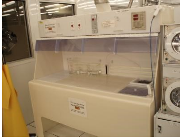
Figure 4-2 Wet deck at the University of Alberta, used for piranha preparation [156].
