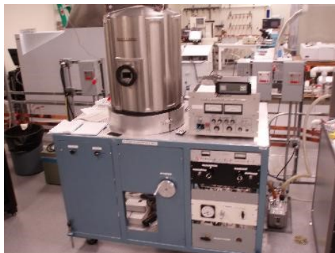
Figure 4-8 Electron beam evaporation system at nanoFAB, University of Alberta [156].
