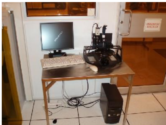
Figure 4-12 First 10 Å contact angle measurement system at nanoFAB, University of Alberta [156].
