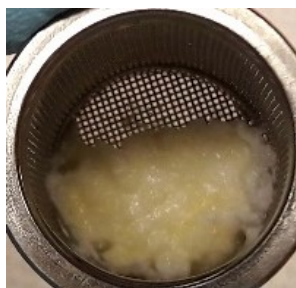
Figure 9.8. Phenytoin sodium and lactose capsules after the dissolution tests. After 30 minutes at body temperature (37.0°C) the capsules became yellow.
