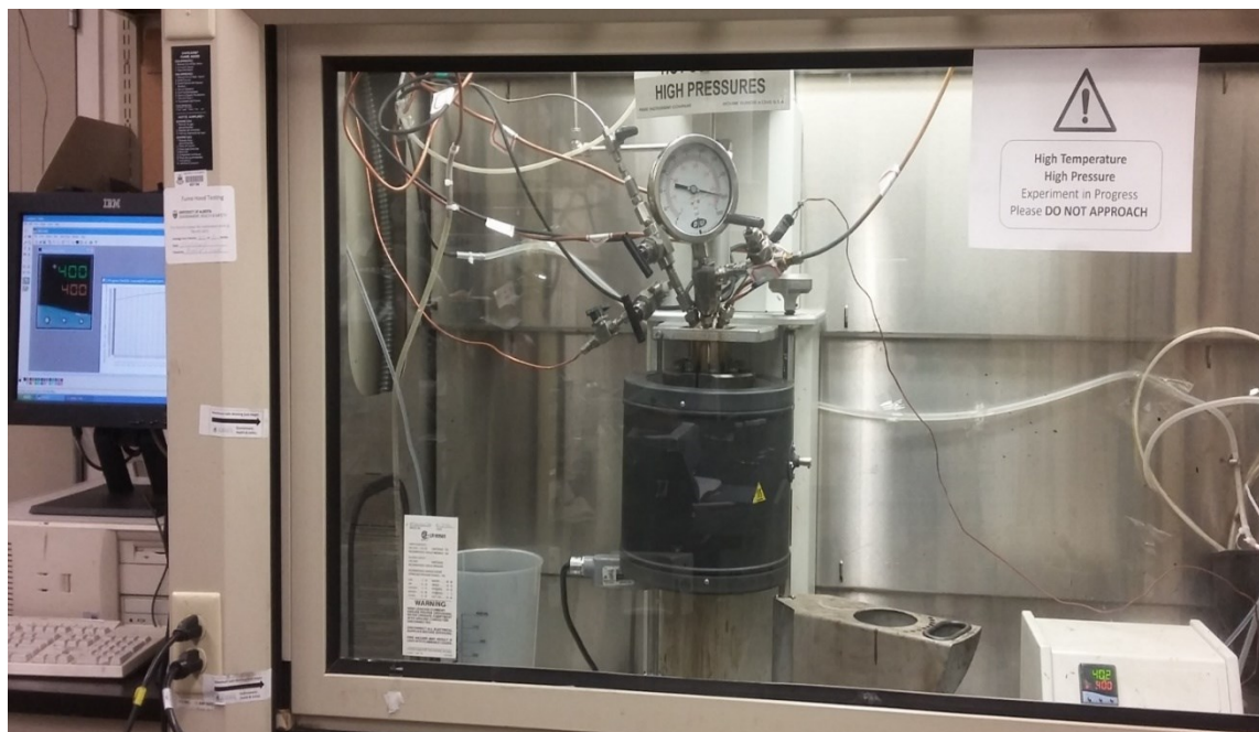
Figure 7 In-lab HTL set-up with controller system
