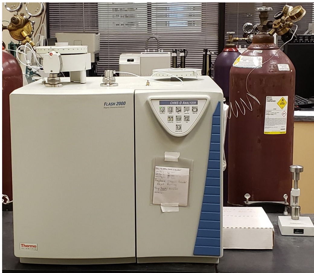
Figure 12 Elemental analysis: Thermo fisher FLASH 2000
