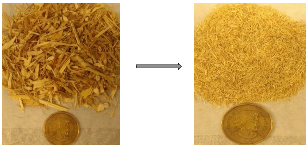
Figure 6 Corn stover reduction from > 9mm to 0.425 – 1 mm
