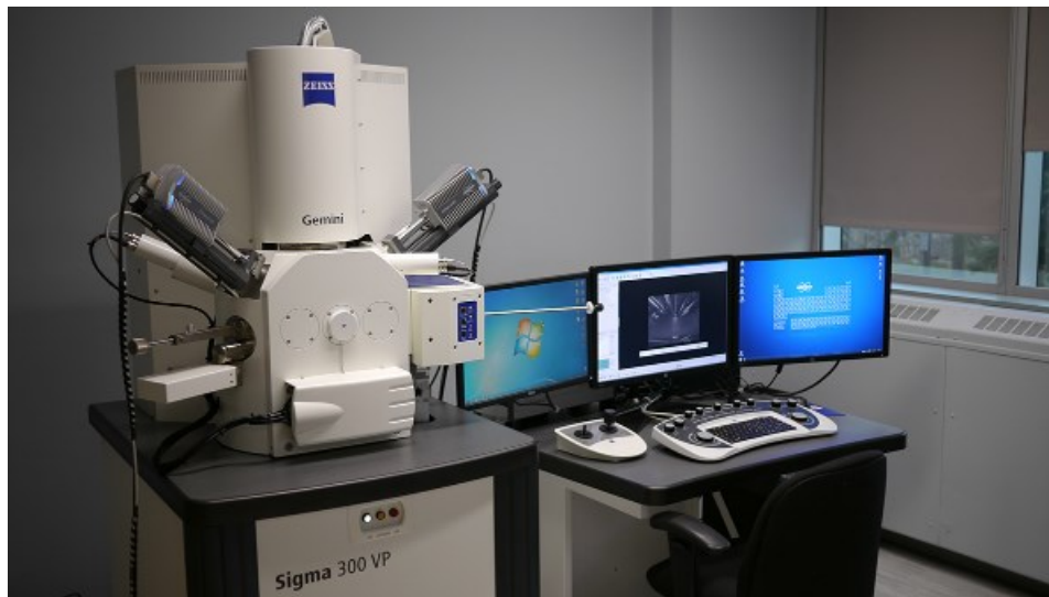
Figure 15 Scanning Electron Microscope Zeiss Sigma 300 VP-FESEM
