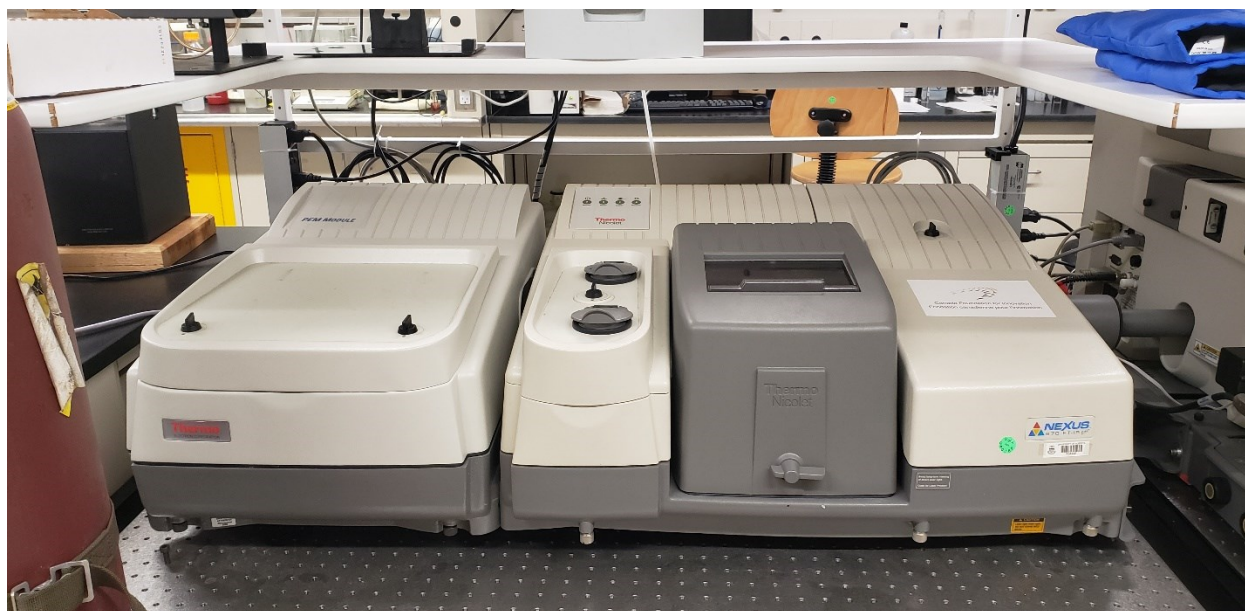
Figure 14 Diffuse Reflectance Thermo NEXUS 870 FTIR
