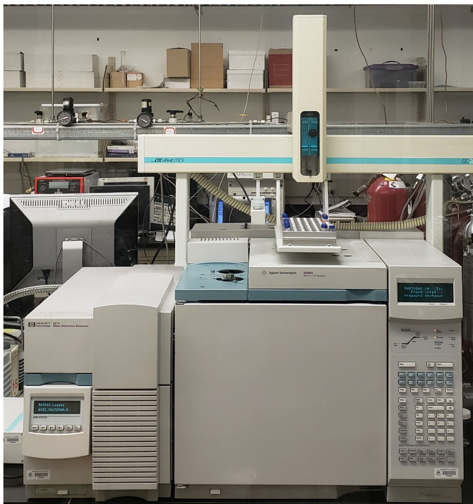
Figure 13 GC-MS analysis: GC (Agilent Technologies 6890N - MS (HP 5973 MSD)
