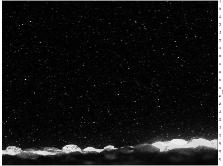
Figure 2-9 A typical PIV image.
