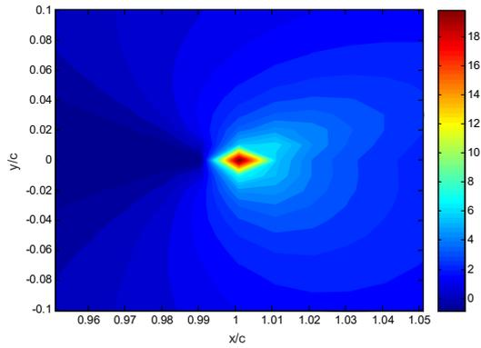
Figure 3. Normalized stress  $\sigma_{yy}/P_0$  around the tip of an interface crack between PZT-4 and SMC.
