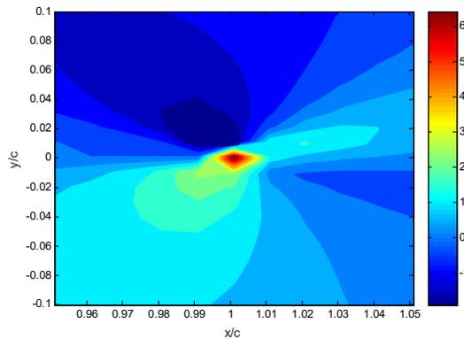
Figure 4. Normalized shear stress  $\sigma_{xy}/P_0$  around the tip of an interface crack between PZT-4 and SMC.
