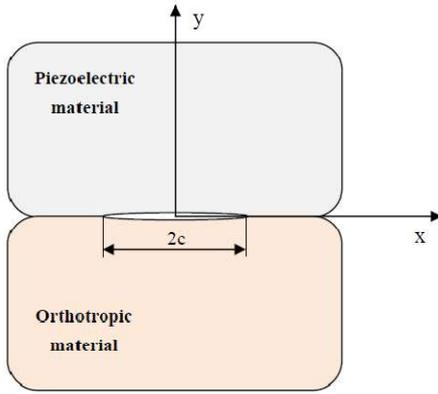
Figure 1. An interface crack between piezoelectric and orthotropic materials.
