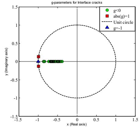
Figure 2.  $g$ -parameter for the interface crack between piezoelectric and orthotropic materials.
