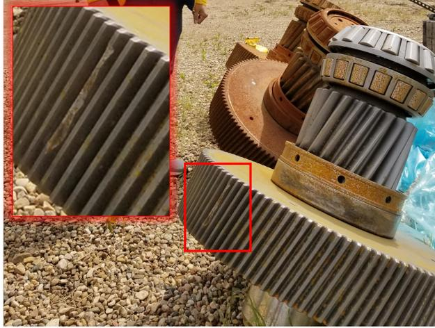
Figure 1.5: Example faulty gear with a broken tooth in Halkirk wind farm, Alberta, Canada. Photo taken by the author in 2019.
