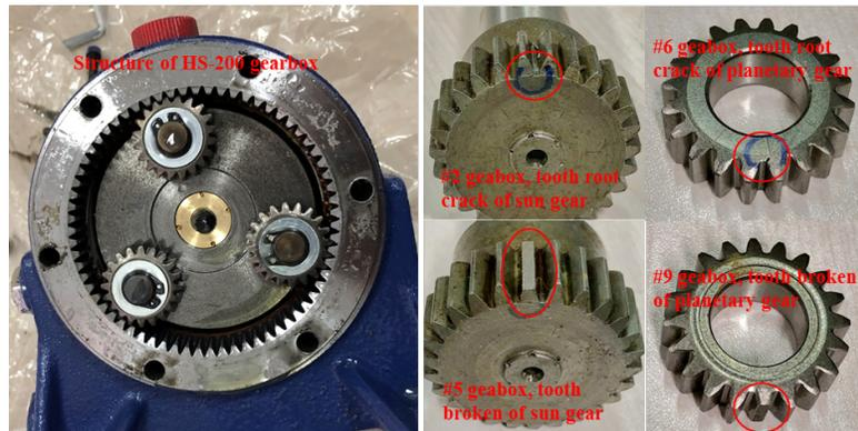
Figure 3.3: Structure of the HS-200 planetary gearbox and 4 example damaged gears.
