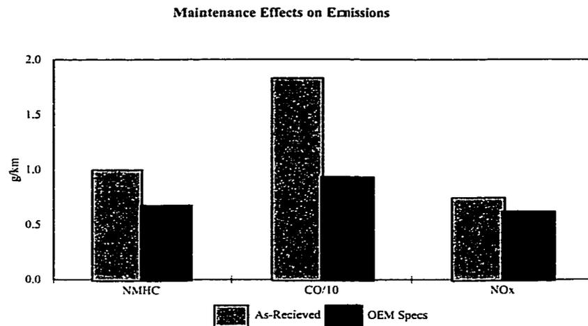
**Figure 2.5: Maintenance Effects on Vehicle Emissions [17]**
