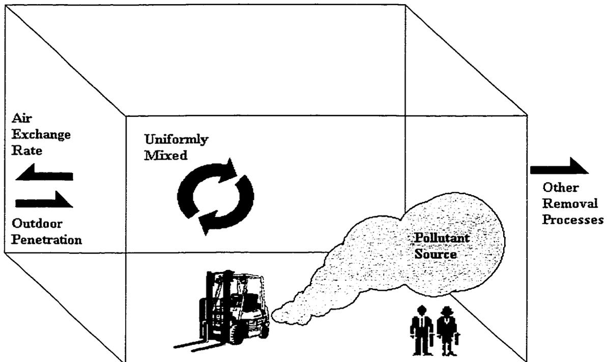
**Figure 4.1: Schematic of a Well Mixed Volume with an Emission Source and Key Parameters.**
