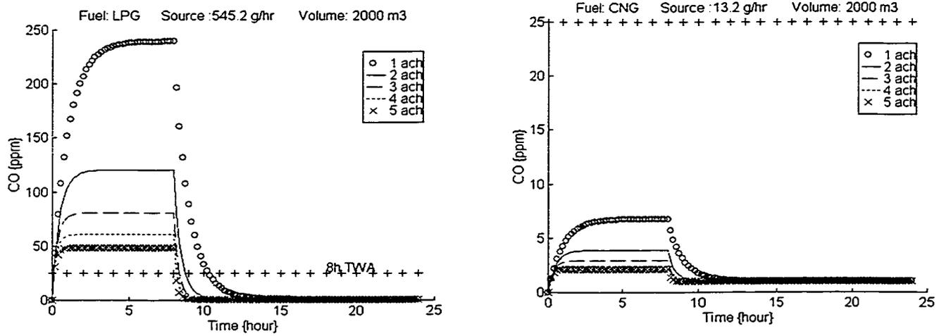
**Figure 4.2: Comparison of Indoor CO Levels with a LPG Forklift and CNG Forklift.**
