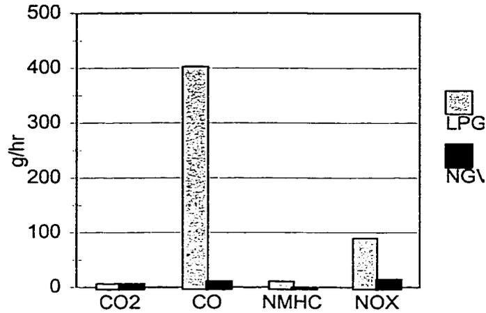
**Figure 3.4: Comparison of Closed Loop CNG Emissions with LPG As-Is Emissions[9]**
