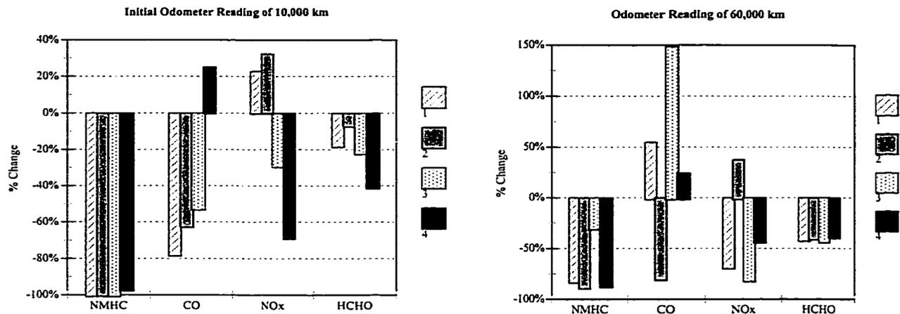
**Figure 2.4: Effect of Mileage Accumulation on Relative Emissions Index for Four Different CNG Conversion Systems, (Emissions Shown as % Change Relative to Gasoline Baseline: Low Mileage and After 60,000 km) [15]**
