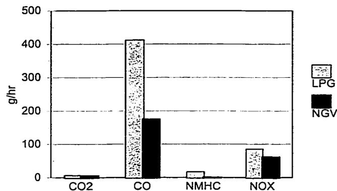
**Figure 3.7: Engine-out Emissions of LPG As-Is and CNG Closed Loop[9]**
