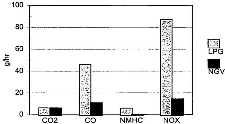
**Figure 3.3: Comparison of Closed Loop CNG Emissions with LPG OEM Emissions[9]**
