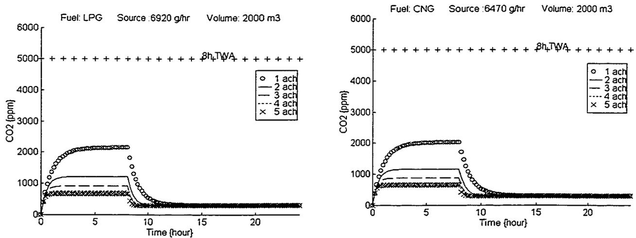
**Figure 4.4: Comparison of Indoor CO<sub>2</sub> Levels with a LPG Forklift and CNG Forklift**
