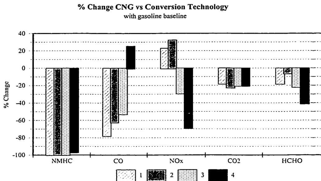
**Figure 2.3: Emissions on CNG Relative to Gasoline for Four Different Conversion Technologies [15]**
