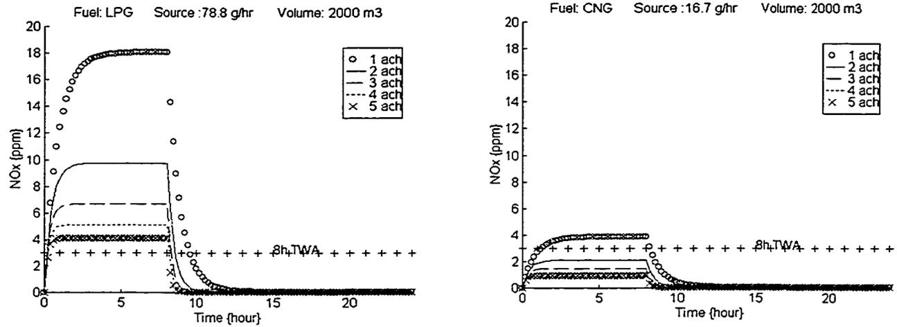
**Figure 4.3: Comparison of Indoor NO<sub>x</sub> Levels with a LPG Forklift and CNG Forklift.**
