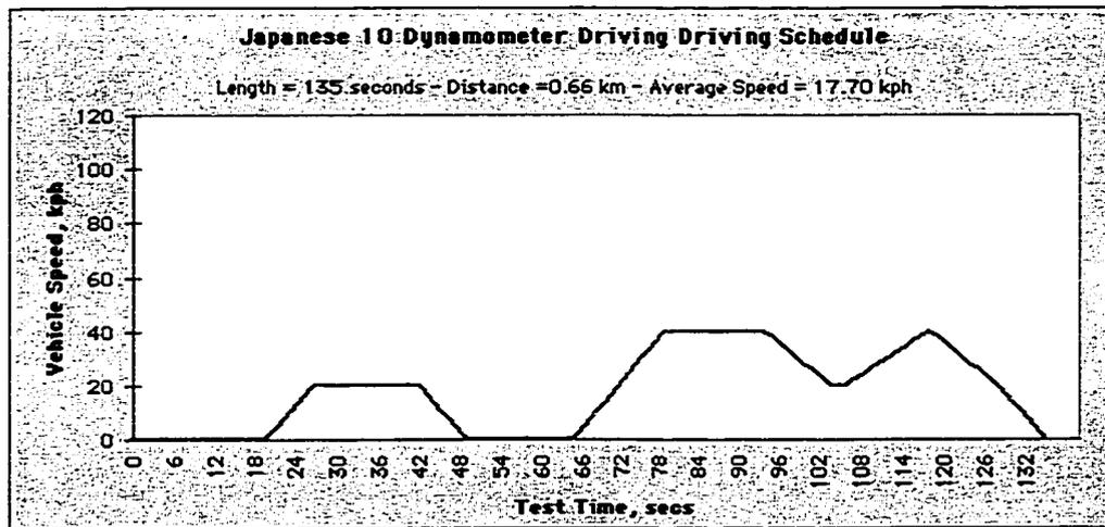
Figure B13: Japanese 10 Mode Test Cycle [2]
