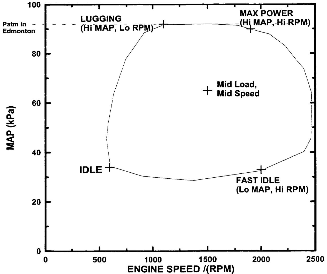
**Figure E1: Typical Operating Range Diagram for Spark Ignition Engine**
