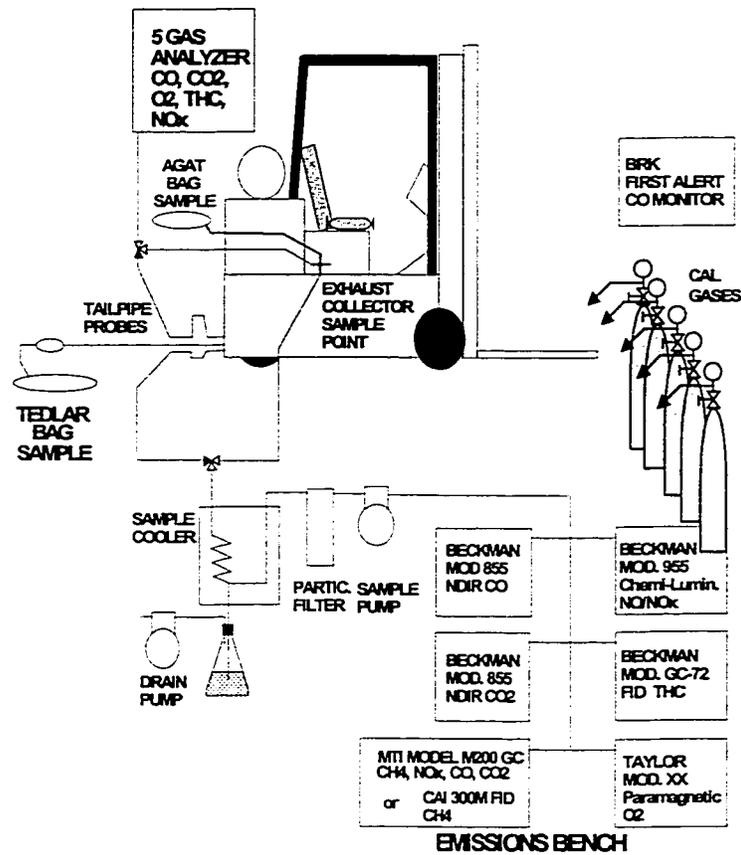
**Figure 3.2: Schematic of Emissions Sampling and Analysis Equipment [9]**
