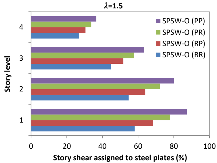
Figure 5.7 Comparison of story shear resisted by steel plates for 4-story SPSW-O systems (no RBS connections)
