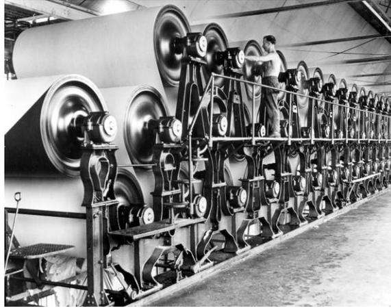
Figure 2.1: Industrial paper making machine (adapted from Flickr (2009))
