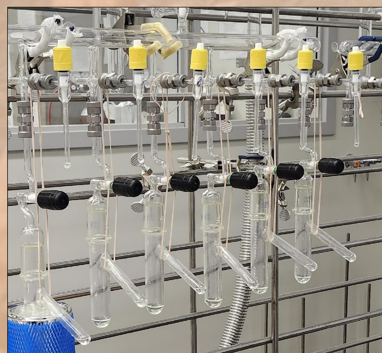
Fig. 4: After the phosphoric acid and CaCO 3 react, the CO 2 gas produced is separated (inside tubes).
