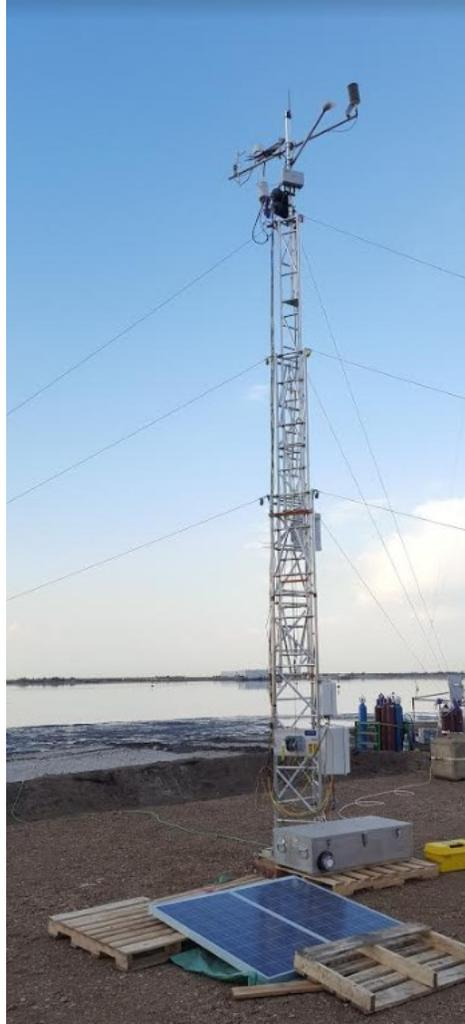
**Figure 4.3. Photo of operating EC system and entire tower with guy wires.**
