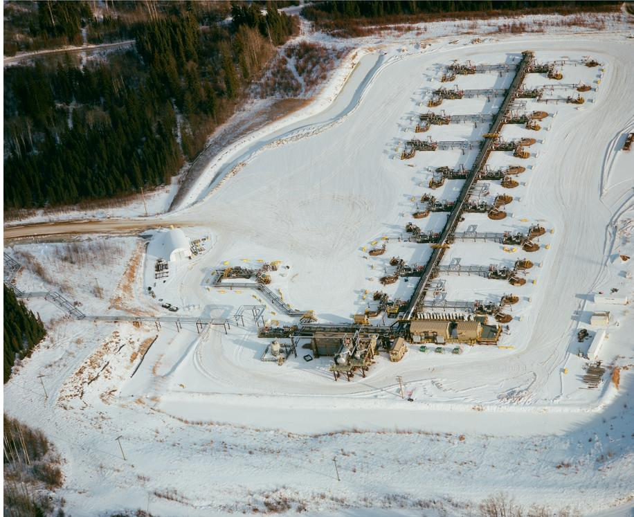
Figure 1.2: Multiple well-pads are set up in lease area, each well-pad has multiple well pairs associated with them as seen from the branched structure from the main line. The figure is obtained from: [link-picture](#), and is available to be reused.
