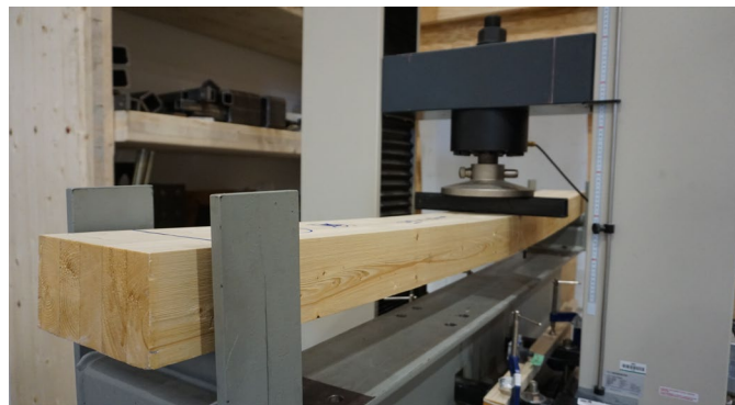
Fig. A3.1 Three-point bending test on a timber beam
