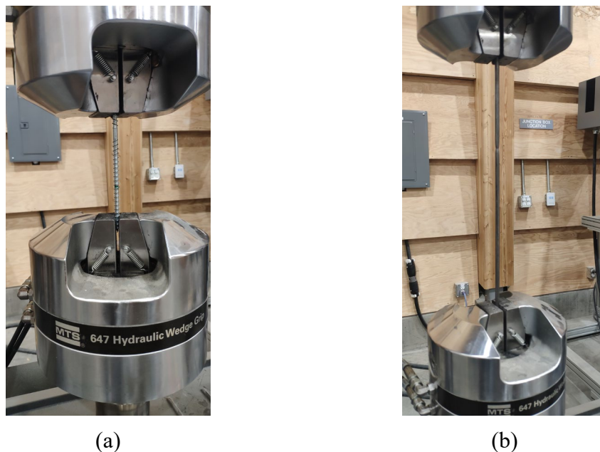
Fig. A5.1 Tensile tests on (a) Self-tapping screws and (b) Steel rods
