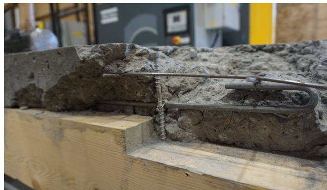
Fig. 4.19 Exposed screw and steel rod in specimen SPR-1 after being tested
