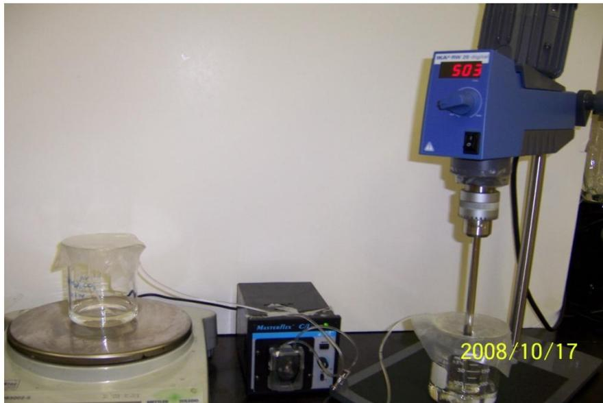
**Figure 3.1 Set-up for colloid preparation.**
