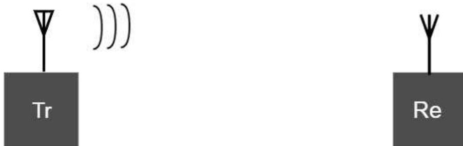
Figure 2.7: SISO system model.
