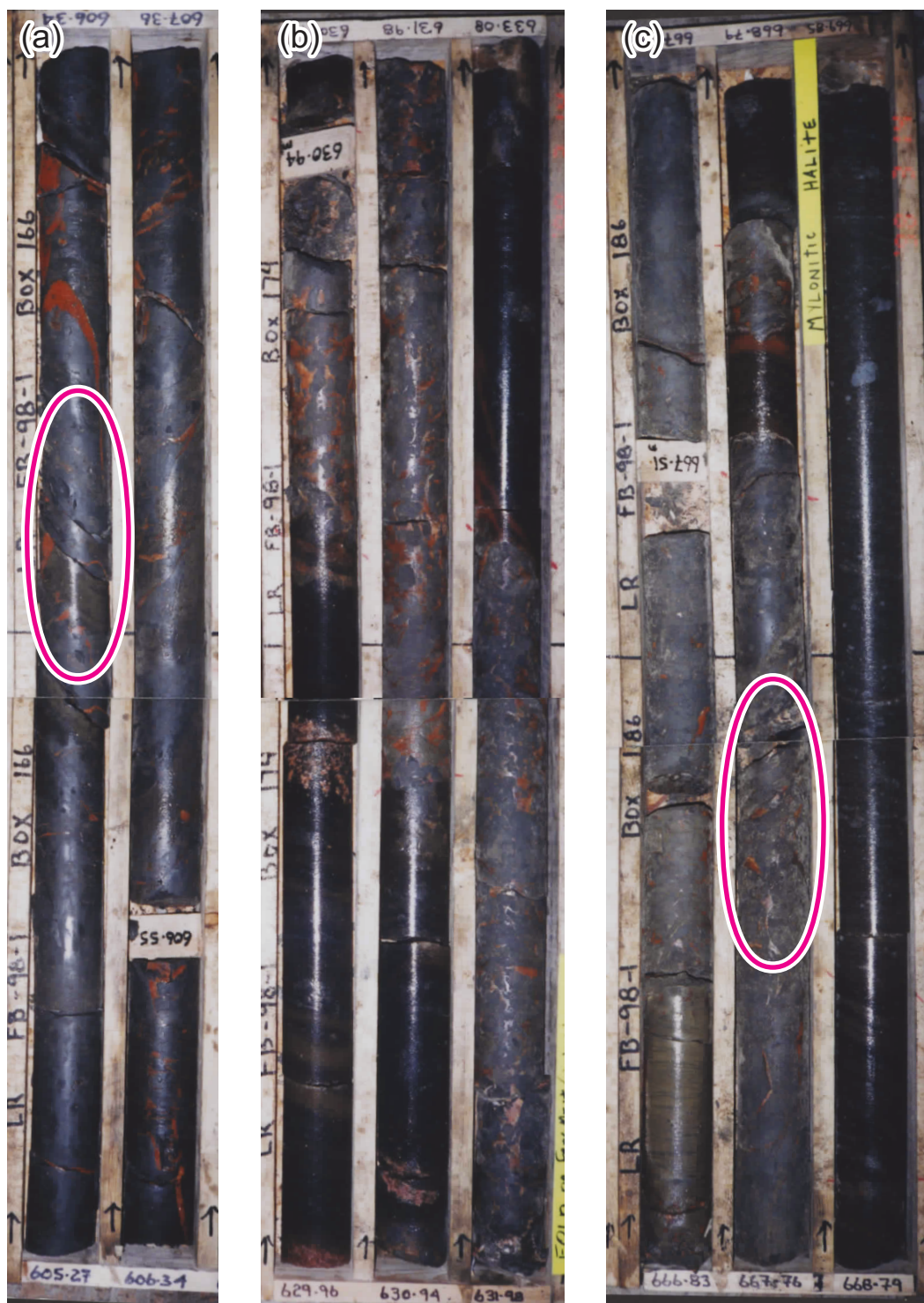
Figure 3.5. Core photograph from LR-98-1 showing dominantly halite and mudstone showing different breccia textures and ratios of halite to mudstone increasing with depth:
