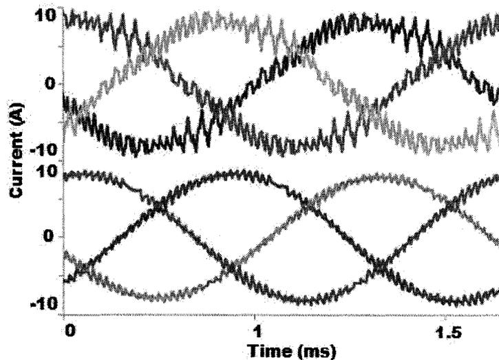
Figure 57: Experimental 18,000 rpm induction motor three phase currents for: standard six switch inverter (upper) and six-switch multi-level inverter (low), with  $m_A = 0.9$ ,  $f_c = 20$  kHz
