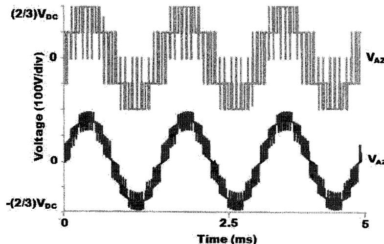
Figure 42: Simulated star connected phase voltage of SS (grey) and SSML topologies with respect to load neutral, z, under DPWM1
