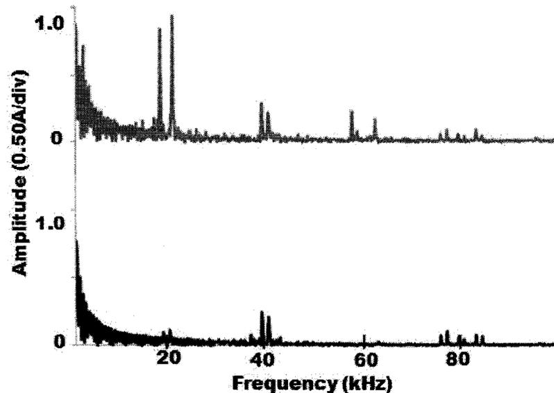
Figure 65: Harmonic spectrum of the motor phase current for: standard six-switch inverter (grey) and three limb SSML topology (black) under DPWM1,  $m_A = 0.9$ ,  $f_c = 20$  kHz
