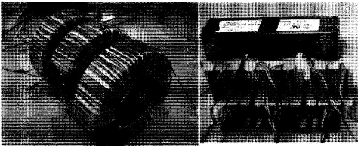
Figure 51: Separate core toroids with split-wound structure (left) and combined three-limb split-wound structure (right)
