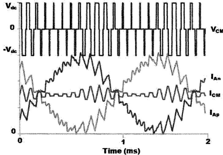
Figure 27: Simulated common mode voltage across inductor and common-mode current with upper and lower winding currents
