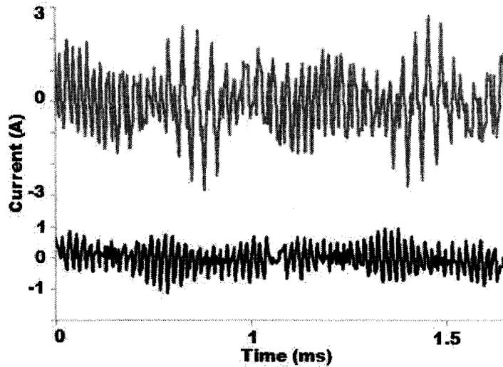
Figure 58: High frequency current ripple for standard six-switch inverter (grey) and separate wound SSML topology (black) under SVPWM,  $m_A = 0.9$ ,  $f_c = 20$  kHz
