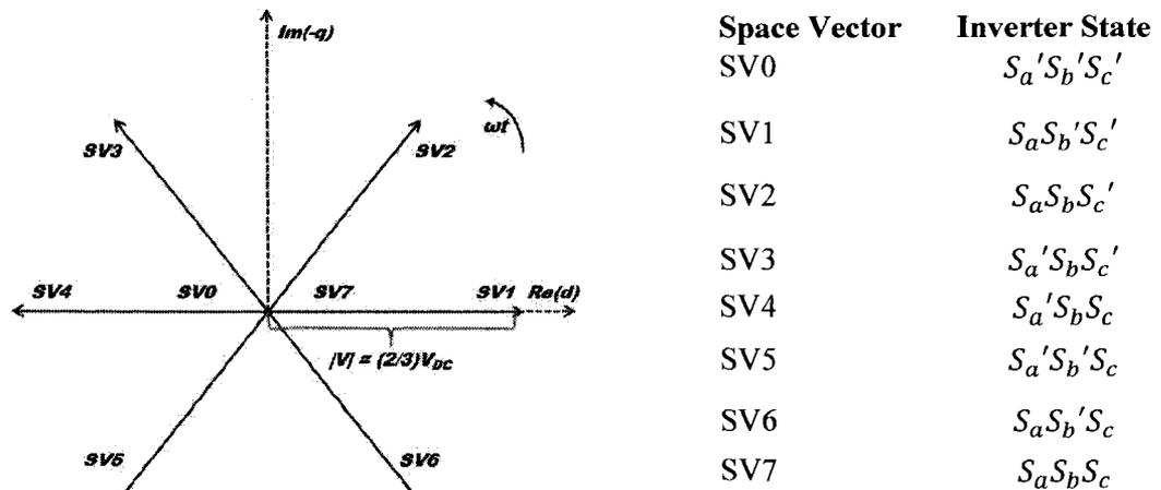
Figure 11: Inverter outputs on the Re-Im plane and the corresponding inverter states with  $S_x$  and  $S_x'$  corresponding to the upper switch on or off respectively for phase 'x' where  $x = a, b, \text{ or } c$
