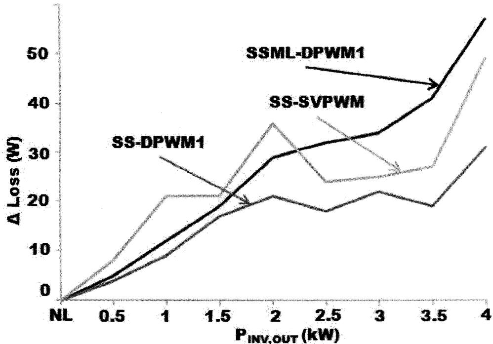
Figure 73: Change in inverter loss with respect to power level: space vector and discontinuous modulation and the SSML topology with discontinuous modulation at  $m_A = 0.9$ ,  $f_c = 20$  kHz
