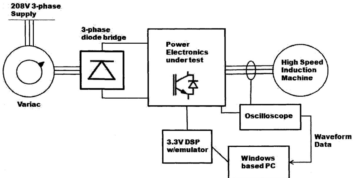
Figure 43: Block Diagram of experimental setup
