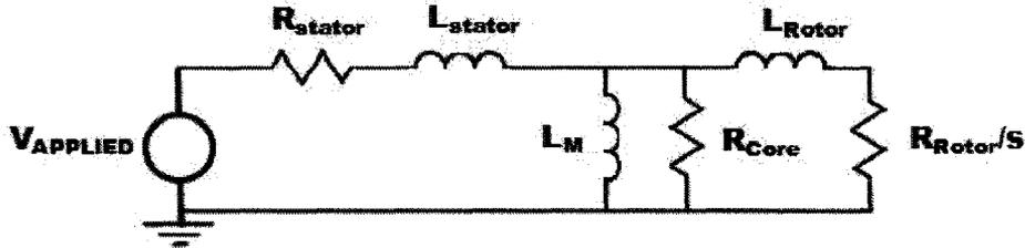
Figure 1: Equivalent per-phase electrical model of an induction motor
