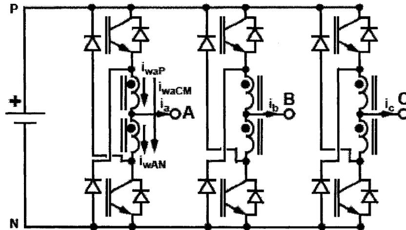
Figure 22: Six-switch Multi-level Inverter topology
