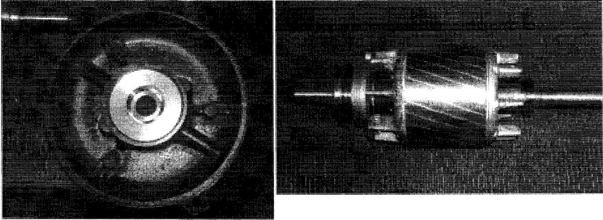
Figure 54: (left) new bearing housing and (right) rotor before balancing
