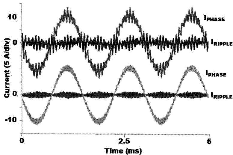
Figure 39: Simulated high frequency ripple comparison: six-switch inverter (top) and multi-level six-switch inverter (bottom) with: SPWM,  $m_A = 0.9$ ,  $m_F = 21$
