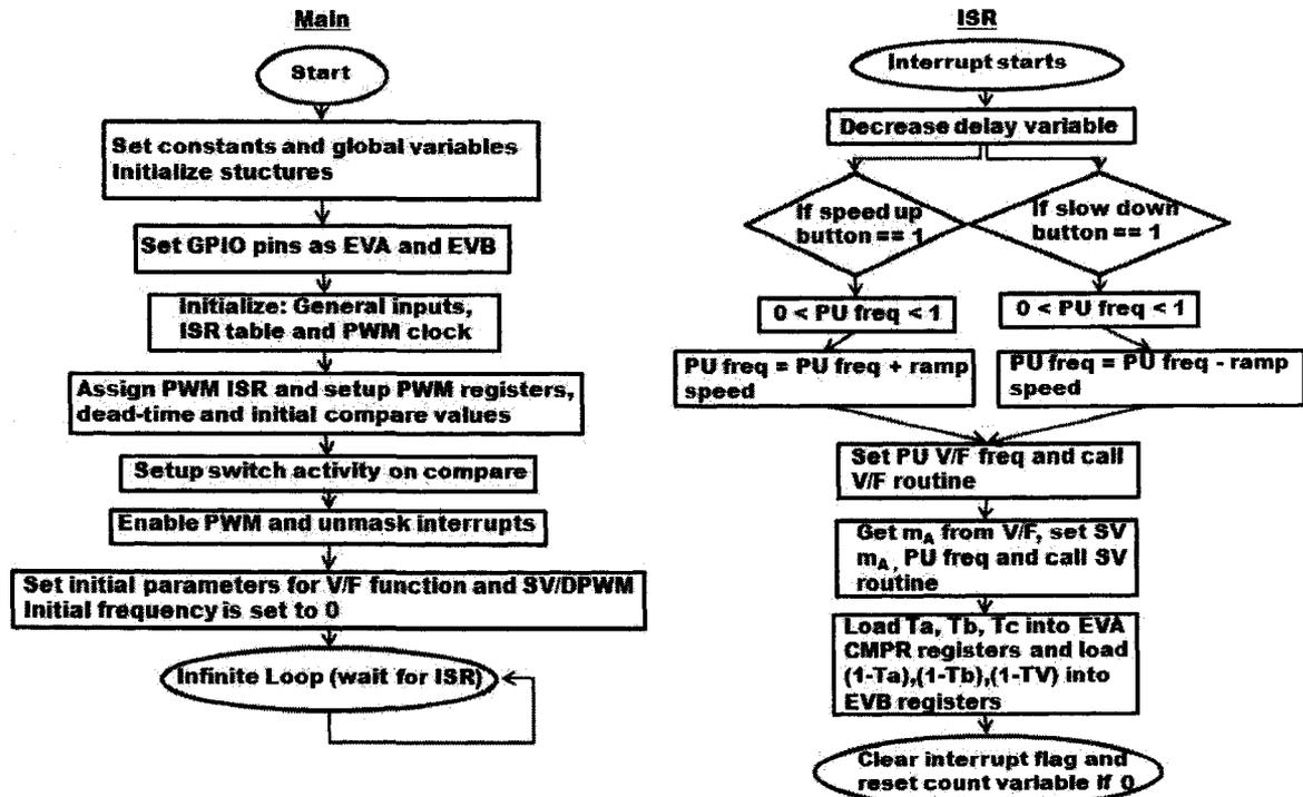
Figure 49: Main code and ISR code block diagrams
