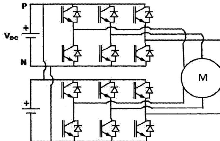
Figure 20: Parallel six-switch inverters with dual three phase windings
