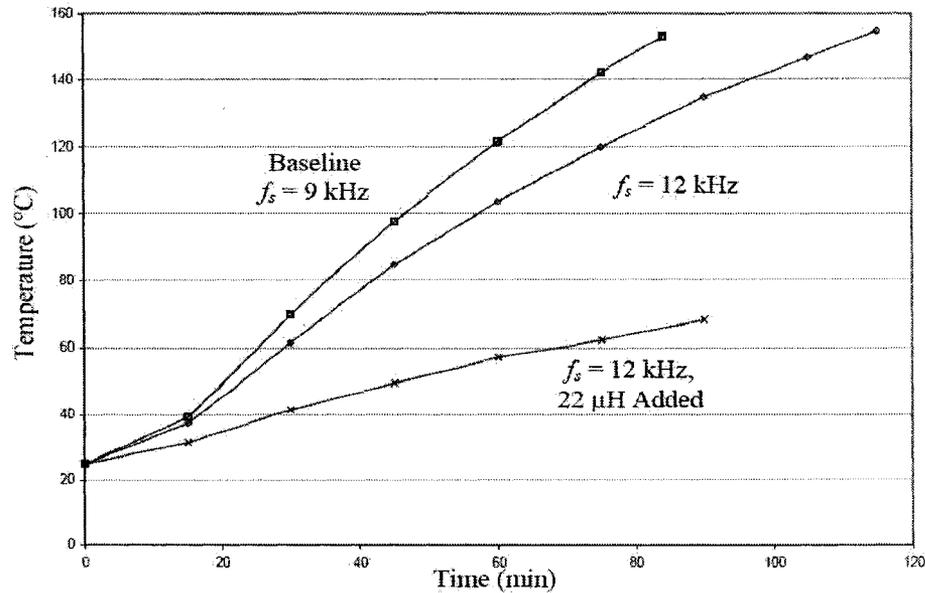
Figure 16: Rotor temperature and various switching frequencies along with a series inductance [13]
