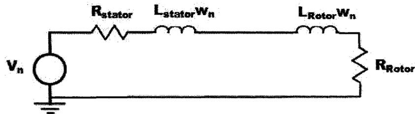
Figure 8: Equivalent circuit for an induction machine considering only the harmonics
