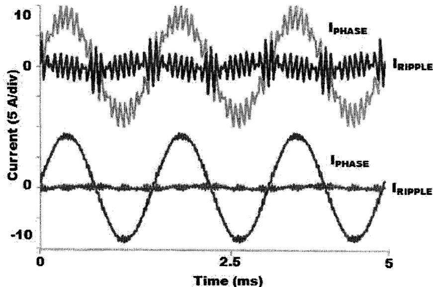
Figure 41: Simulated high frequency ripple comparison: six-switch inverter (top) and multi-level six-switch inverter (bottom) with: DPWM1,  $m_F = 21$  with inductive current demand of 10A peak
