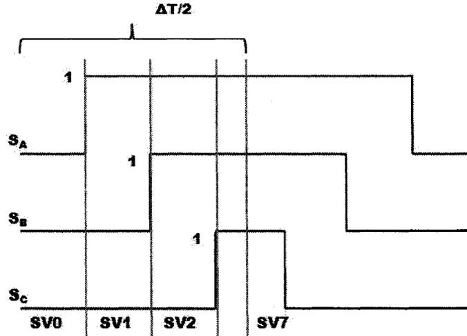
Figure 12: Space vector switching example with  $m_A = 0.5$  and a phase angle of  $30^\circ$
