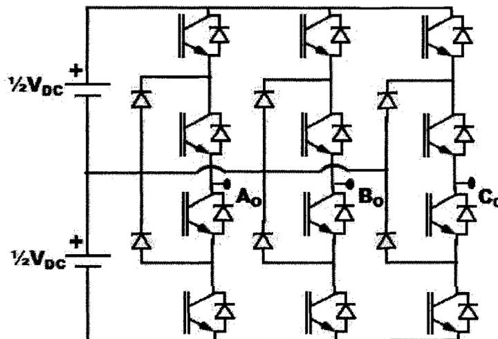
Figure 19: Three Level Neutral Point Clamped Inverter Topology
