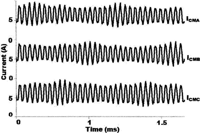
Figure 67: Three phase common mode currents for the combined SSML topology
