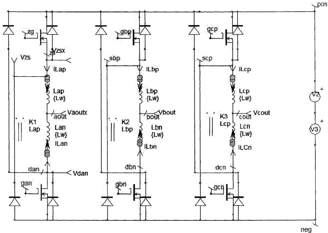
Figure 31: Six-switch Multi-level Inverter spice model
