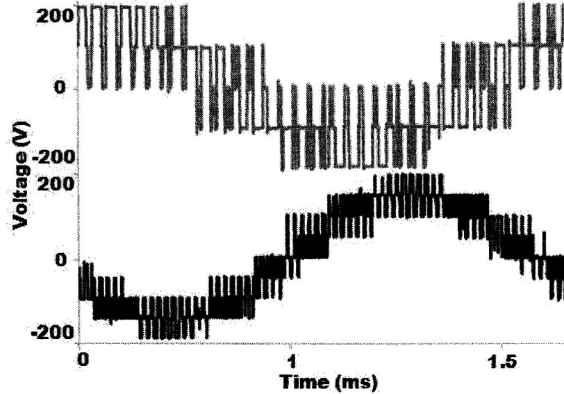
Figure 69:  $V_{AZ}$  for: six-switch inverter (grey) and combined SSML topology (black)
