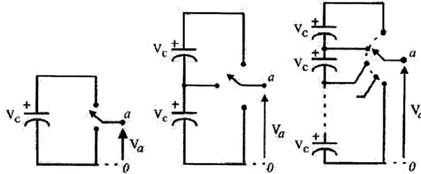
Figure 18: Multilevel inverter states: 2-level, 3-level and n-level [53]
