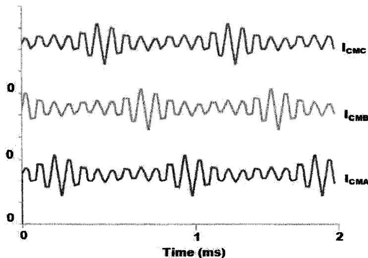
Figure 36: Simulated three phase common mode currents for interleaved DPWM and the combined three limb core for the SSML topology
