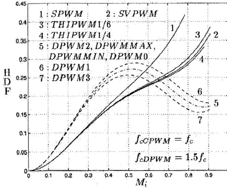
Figure 14: A graphical illustration of the various switching methods from [29], where HDF indicates a harmonic distortion factor and  $M_i$  is the modulation depth
