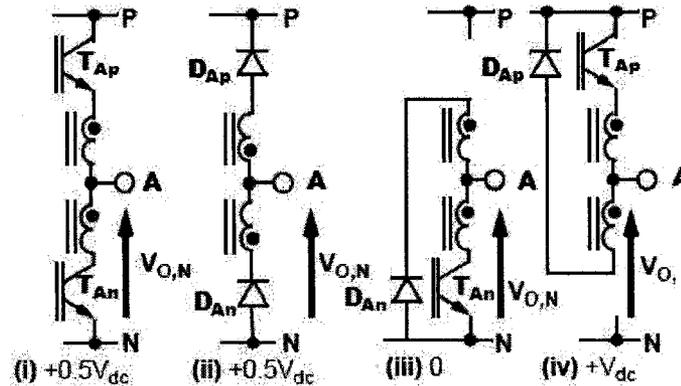
Figure 24: Switch states of the SSML inverter topology
