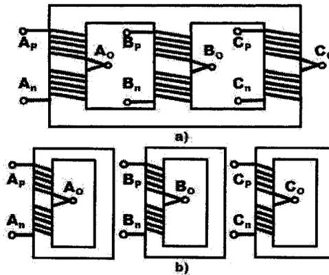
Figure 29: a) combined three limb core b) separate three limb cores
