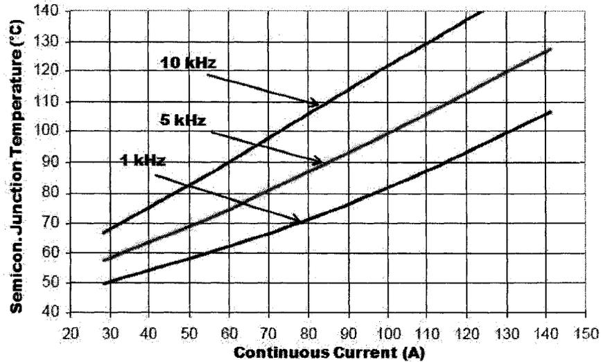
Figure 7: Typical switching characteristics for 100A, 20 kHz rated IGBT module and steady state junction temperature value [16]
