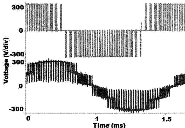
Figure 56: Experimental VAB on 18,000 rpm induction machine: standard six-switch inverter (grey) and six-switch multi-level inverter (black) under SVPWM,  $m_A = 0.9$ ,  $f_c = 20$  kHz
