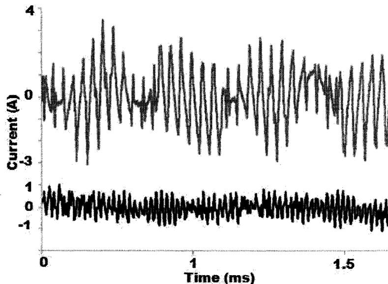
Figure 64: High frequency current ripple of unloaded 18,000 induction motor with standard six-switch inverter(grey) and combined core SSML topology(black) under DPWM1,  $m_A = 0.9$ ,  $f_c = 20$  kHz
