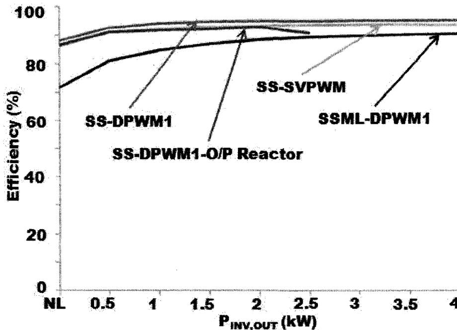
Figure 71: Efficiency of six-switch with: space vector and discontinuous modulation and the SSML topology with discontinuous modulation at  $m_A = 0.9$ ,  $f_c = 20$  kHz
