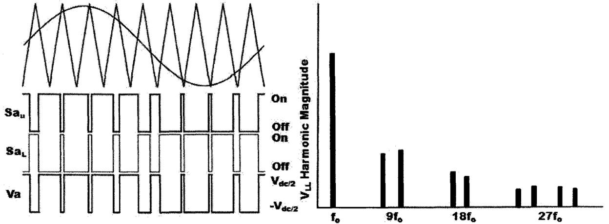
Figure 6: Switching logic and output phase voltage for one inverter leg and the line-line harmonic content from sinusoidal PWM
