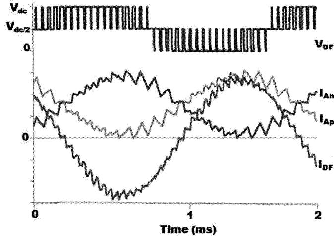
Figure 28: Simulated differential voltage across inductor and differential mode current with upper and lower winding currents
