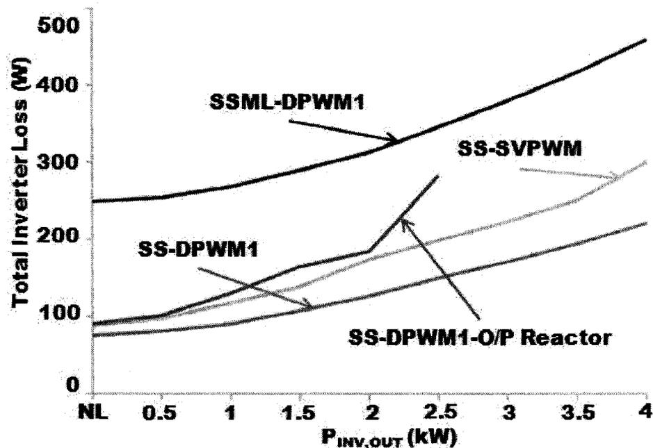
Figure 72: Total inverter loss of six-switch with: space vector and discontinuous modulation and the SSML topology with discontinuous modulation at  $m_A = 0.9$ ,  $f_c = 20$  kHz
