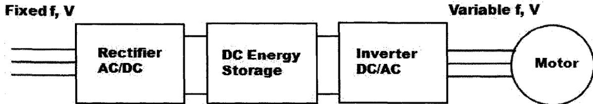
Figure 4: General Conversion to variable frequency and voltage by a variable speed drive
