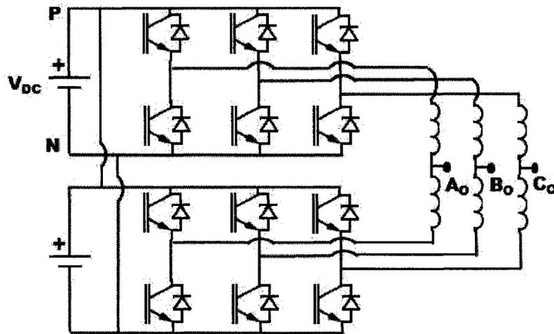
Figure 21: Parallel six-switch inverters with current sharing output reactors
