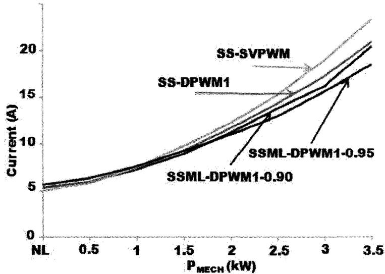
Figure 76: RMS phase current versus output mechanical power at  $m_A = 0.9$  (0.95 for one SSML case)
