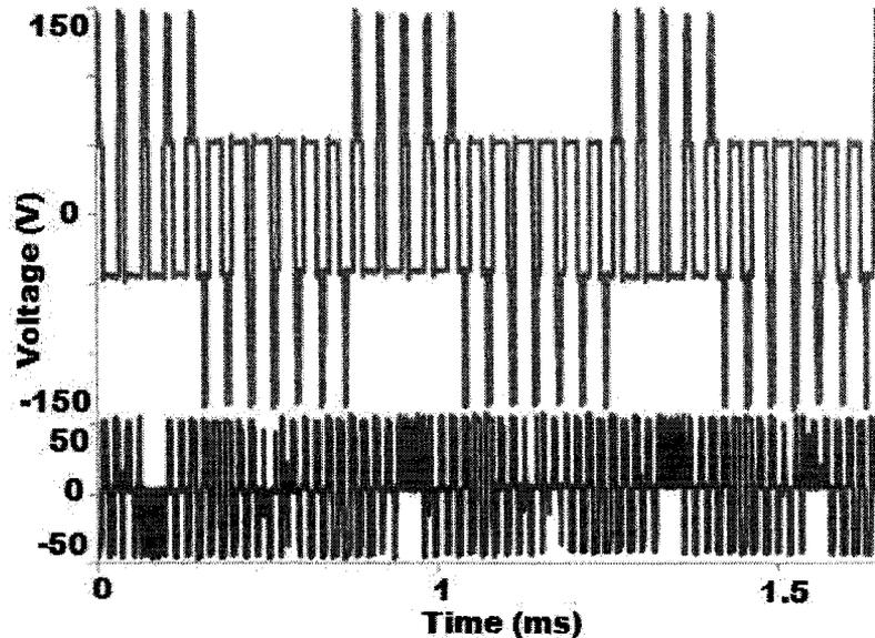
Figure 70:  $V_{NZ}$  : six-switch inverter (grey) and combined SSML topology (black)
