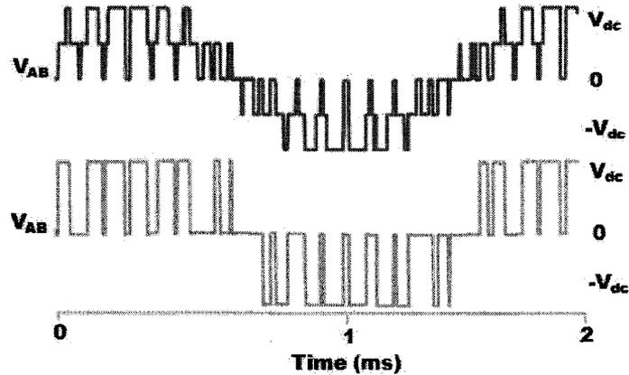
Figure 25: Simulated Line to line PWM outputs of SSML inverter (black) and the standard six-switch inverter (grey) with  $m_A = 0.9$  and  $m_F = 9$
