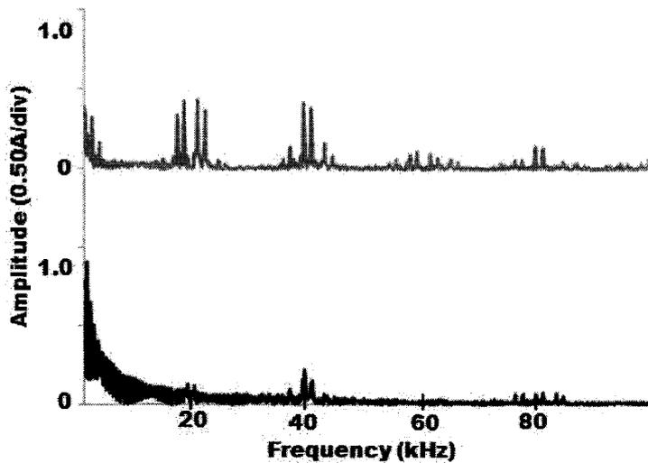
Figure 59: Harmonic spectrum of the motor phase current for: standard six-switch inverter (grey) and separately wound SSML topology (black) under SVPWM,  $m_A = 0.9$ ,  $f_c = 20$  kHz
