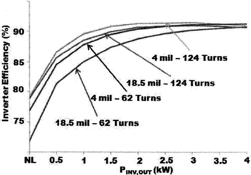
Figure 74: Output Inverter Efficiency with varying lamination size and series connected turns
