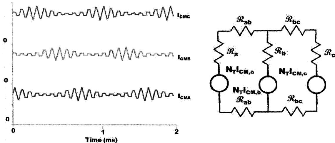
Figure 32: Simulated common mode currents for phase a,b and c under interleaved SPWM and reluctance circuit of three limb core (right)
