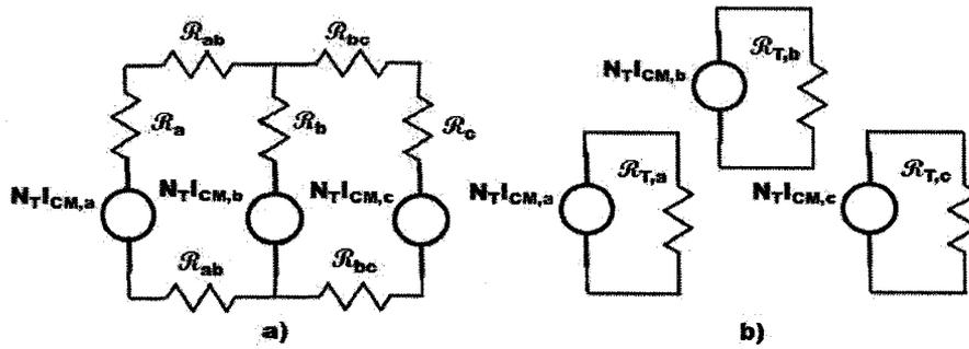
Figure 30: a) combined three limb reluctance circuit b) separate cores reluctance circuit
