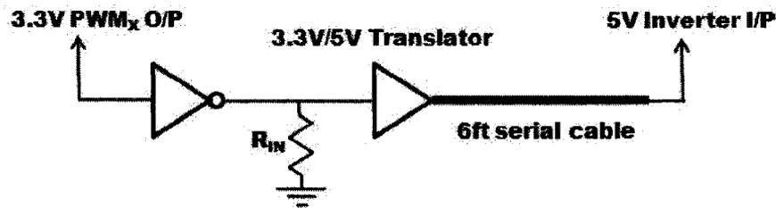
Figure 47: PWM output of DSP to inverter drive circuitry
