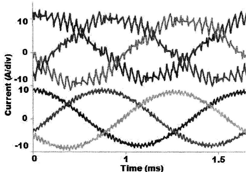
Figure 63: Three phase currents of unloaded 18,000 induction motor with standard six-switch inverter(upper) and combined core SSML topology under DPWM1 (lower),  $m_A = 0.9$ ,  $f_c = 20$  kHz
