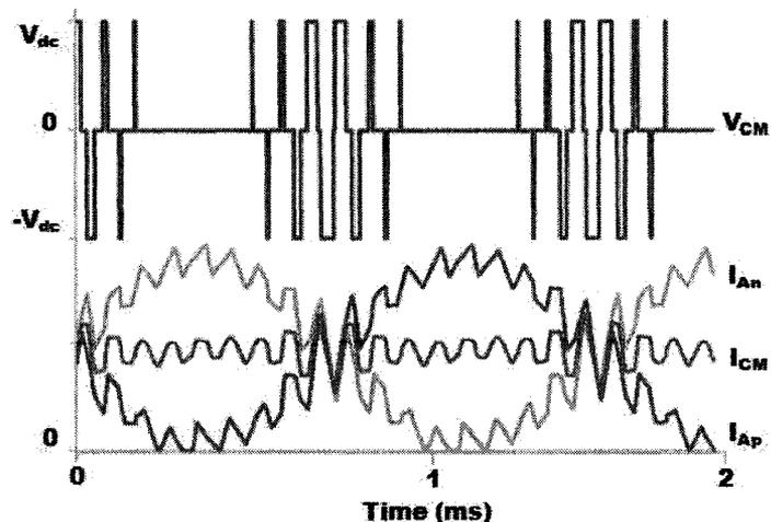
Figure 35: Simulated common mode voltage and winding currents in phase A, under DPWM operation and a three-limb core
