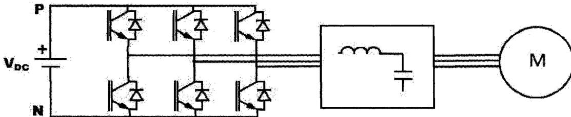
Figure 17: LC or ‘sine wave’ filter in a variable speed drive system
