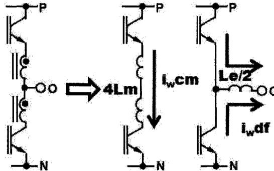
Figure 26: Impedance for common mode and differential mode currents due to the split wound inductor
