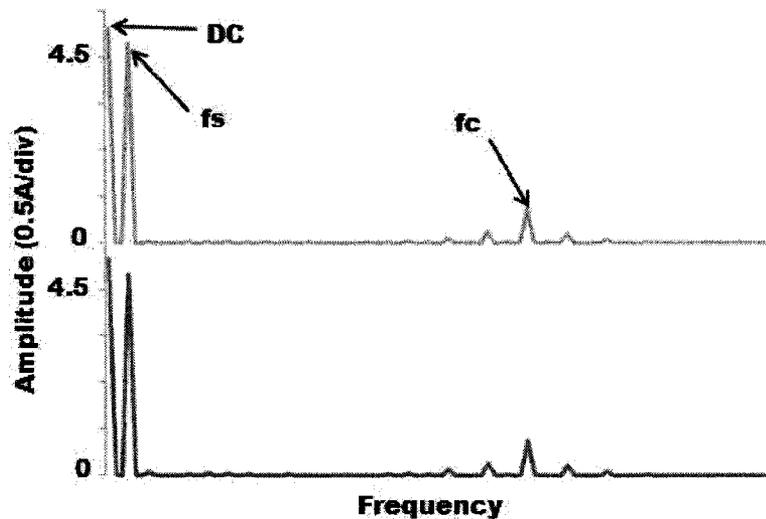
Figure 37: Fourier spectrums of the simulated upper (grey) and lower (black) winding currents
