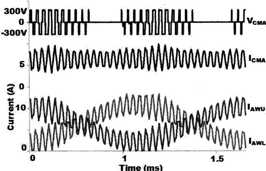
Figure 66: Common mode voltage, current and winding currents for three limb SSML topology under DPWMI,  $m_A=0.9$ ,  $f_c = 20 \text{ kHz}$
