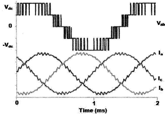
Figure 34: Simulated Line to line voltage of combined three limb core using DPWM1 and corresponding phase currents ( $mF = 18$ )
