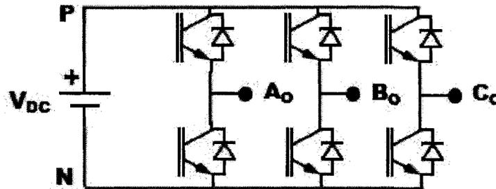
Figure 5: Standard six-switch inverter
