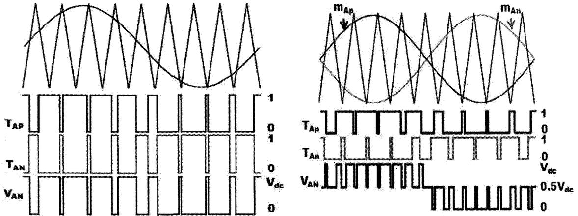
Figure 23: Switch logic and PWM leg output for the six-switch inverter (left) and the six-switch multi-level inverter (right) under sinusoidal PWM (interleaved for SSML), with  $m_A=0.9$  and  $m_f=9$
