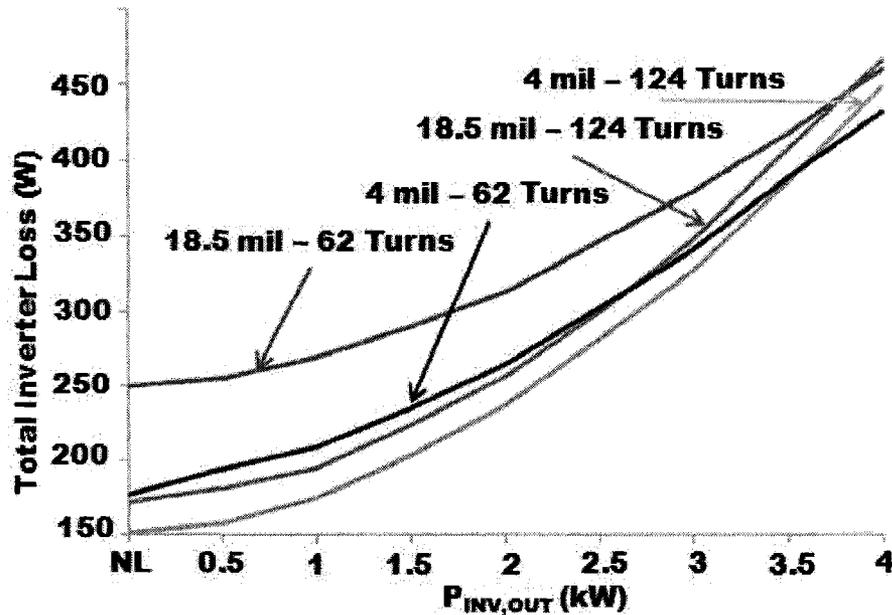
Figure 75: Total inverter losses as a function of changing lamination thickness and series connected turns
