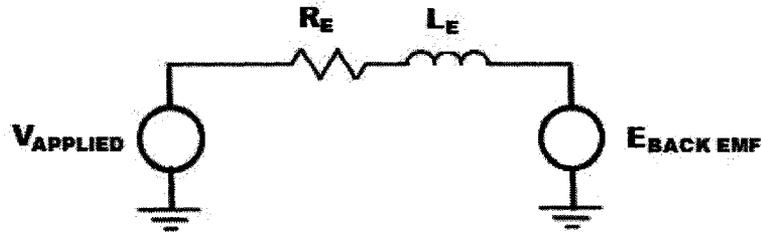
Figure 2: Equivalent circuit for the synchronous machine
