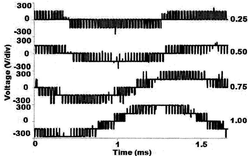
Figure 68:  $V_{AB}$  for various modulation indexes of the combined core SSML topology
