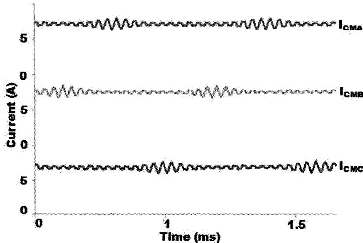
Figure 61: Three phase common mode currents for the separately wound SSML topology
