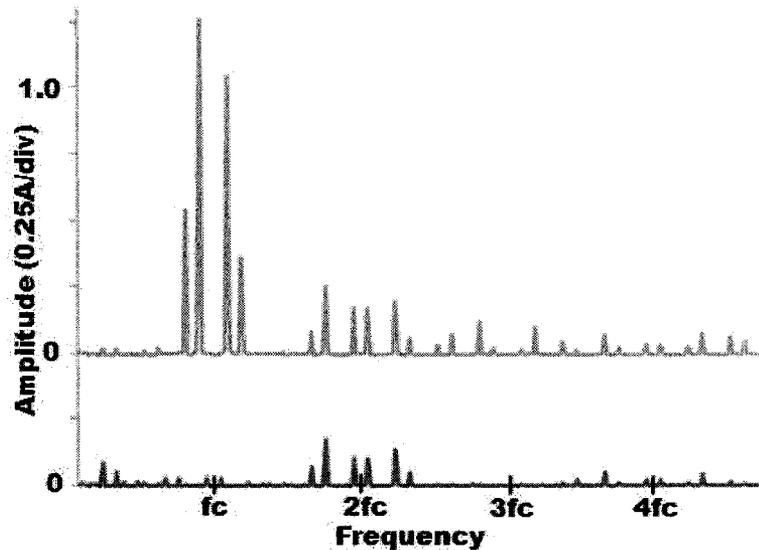
Figure 40: Simulated frequency spectrum of standard six-switch inverter (grey) and SSML inverter under DPWM1,  $m_f = 21$  with the combined core structure
