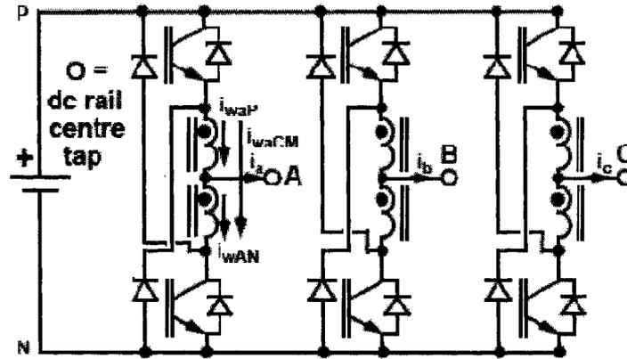
Figure 9: Proposed multi-level topology for high speed drive
