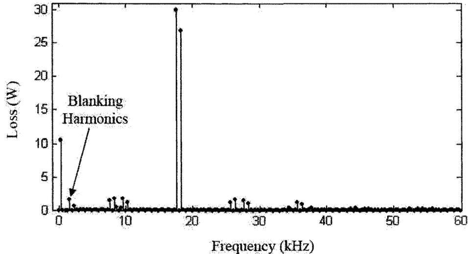
Figure 15: Rotor Loss spectrum density from [13] with a switching frequency of 9 kHz and a blanking time of 3 $\mu$ s
