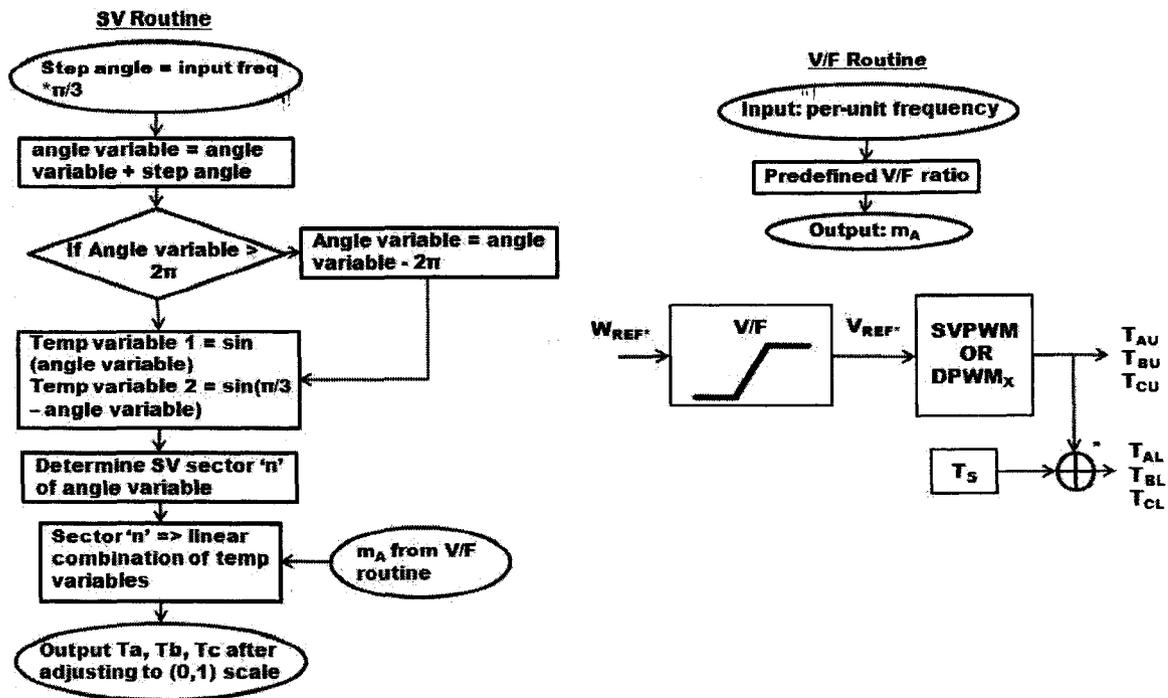
Figure 50: Space vector routine (same for centered or DPWMx) and V/F routine block diagrams
