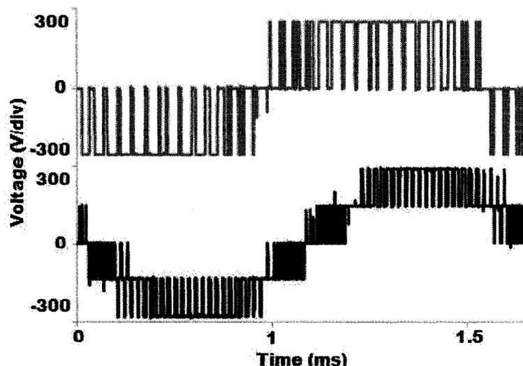
Figure 62:  $V_{AB}$  for six-switch inverter (grey) and combined core SSML topology (black) under DPWMI,  $m_A = 0.9$ ,  $f_c = 20$  kHz
