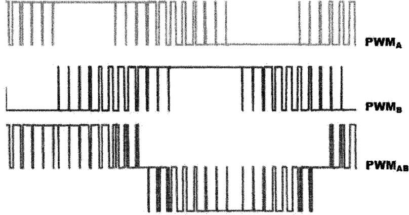
Figure 13: DPWM1 phase A and B PWM voltages and line-to-line PWM voltages over one complete fundamental cycle
