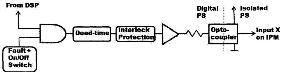
Figure 45: Logic flow of PWM path for a given switch of the inverter
