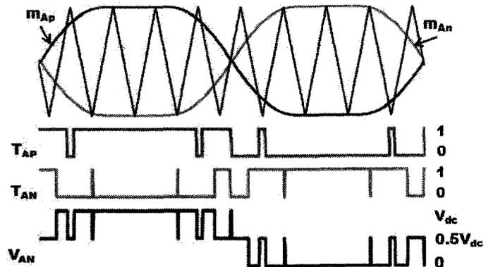
Figure 33: DPWM1 approximate clamping table (left) and PWM switching sequence (right) with combined three limb core and interleaved DPWM ( $m_f = 18$ )
