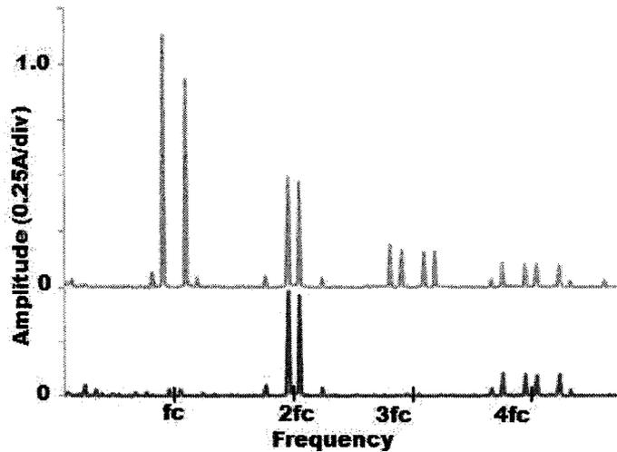
Figure 38: Simulated frequency spectrum of standard six-switch inverter (grey) and SSML inverter under SPWM,  $m_A=0.9$ ,  $m_F=21$  with three separate cores
