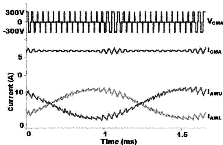
Figure 60: Common mode voltage, current and winding currents for separately wound SSML topology
