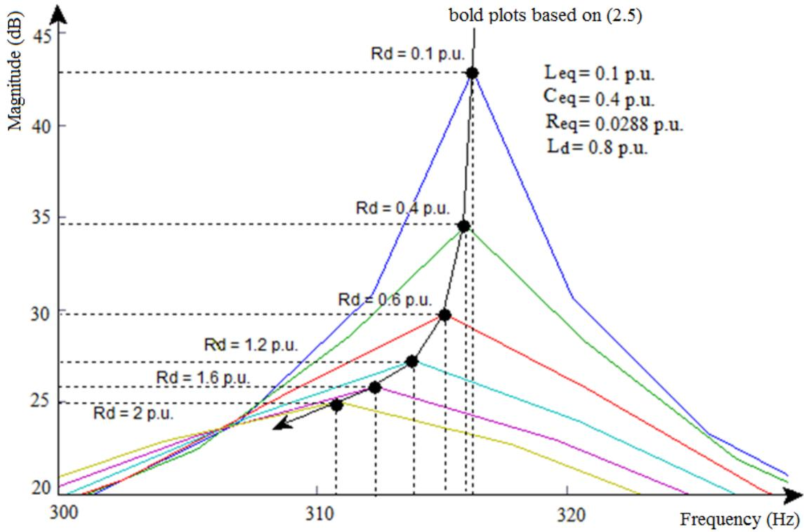
Figure 2.3: Effects of  $R_d$  on the input LC resonance
