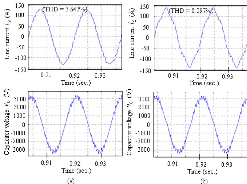
Figure 4.1:  $i_s$  and  $v_c$  of filter design simulation case 1
