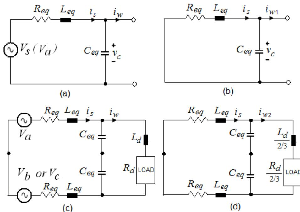
Figure 2.1: Modeling of the effects of CSR DC side circuit
