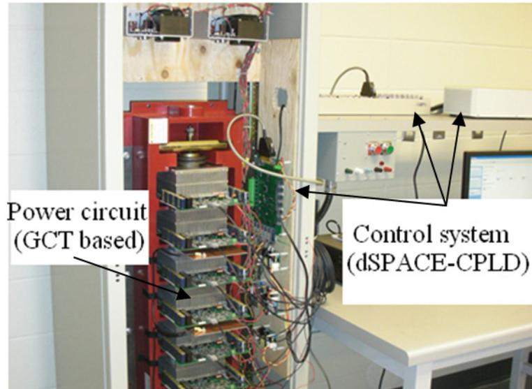
Figure 5.1: Experimental CSR prototype
