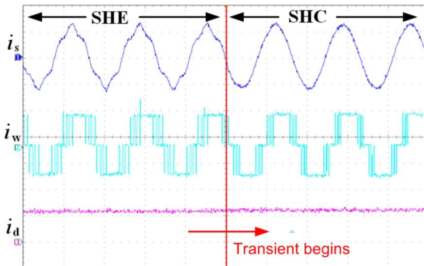
Figure 5.6: Results of SHC experiment case 2
