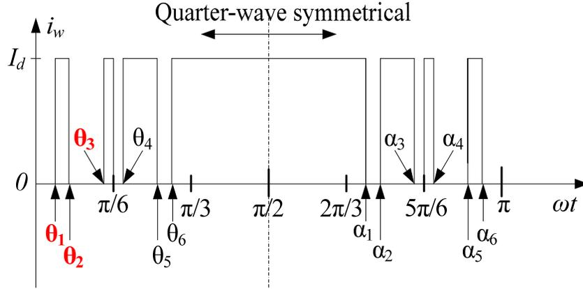
Figure 3.2: Traditional SHE PWM pattern (7 pulses per half cycle)
