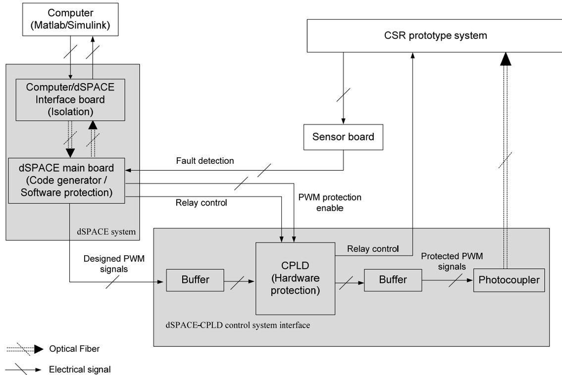
Figure 5.2: dSPACE-CPLD Control system
