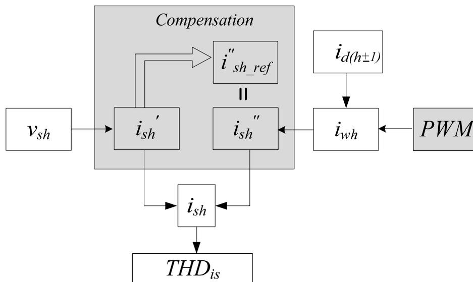
Figure 3.1: Relationship diagram of SHC scheme variables
