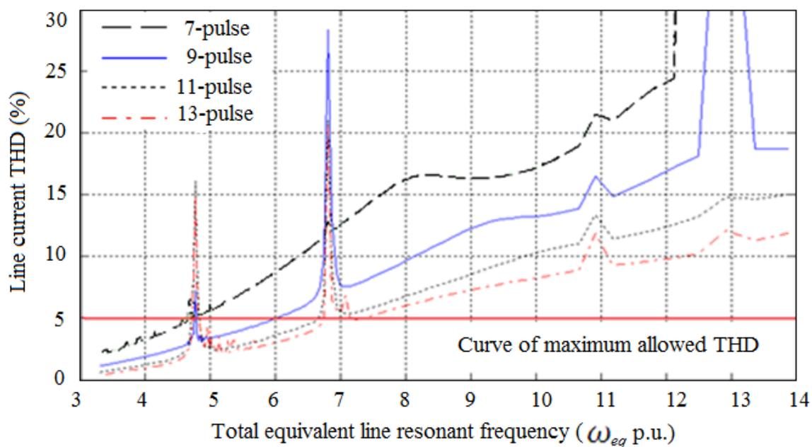
Figure 2.7: THD curves for filter inductor design example
