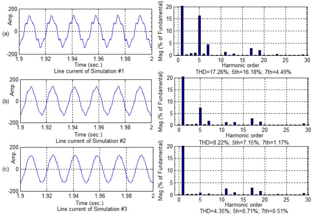
Figure 4.3:  $i_s$  waveforms and spectra of SHC simulations
