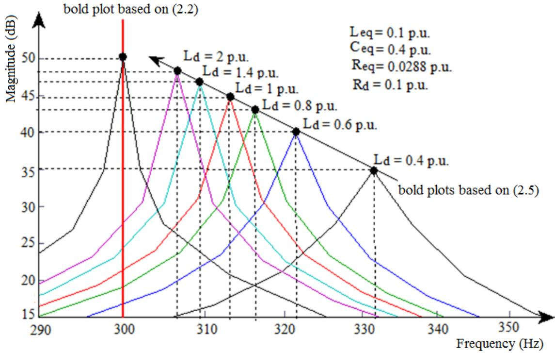
Figure 2.2: Effects of  $L_d$  on the input LC resonance
