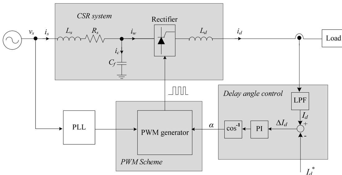
Figure 1.2: Control scheme of a high-power PWM CSR system
