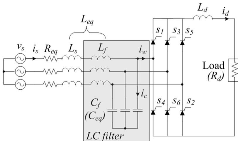
Figure 1.1: Typical circuit of a PWM CSR system
