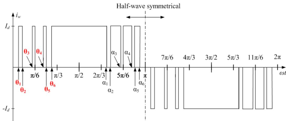
Figure 3.3: PWM pattern for SHC (7 pulses per half cycle)
