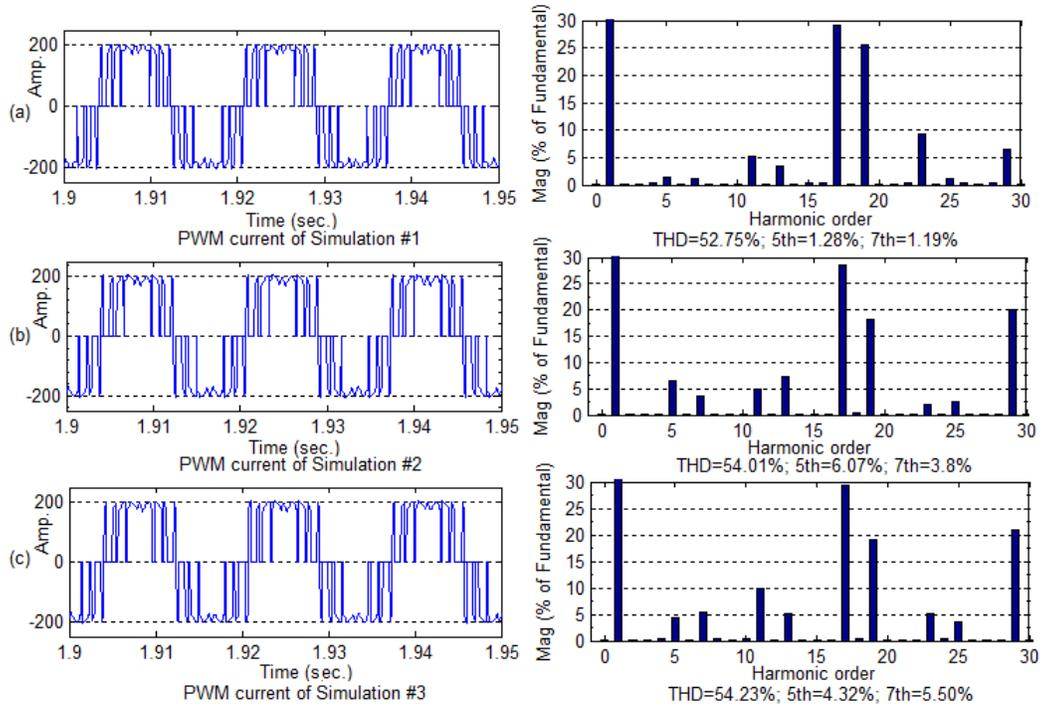
Figure 4.4:  $i_w$  waveforms and spectra of SHC simulations
