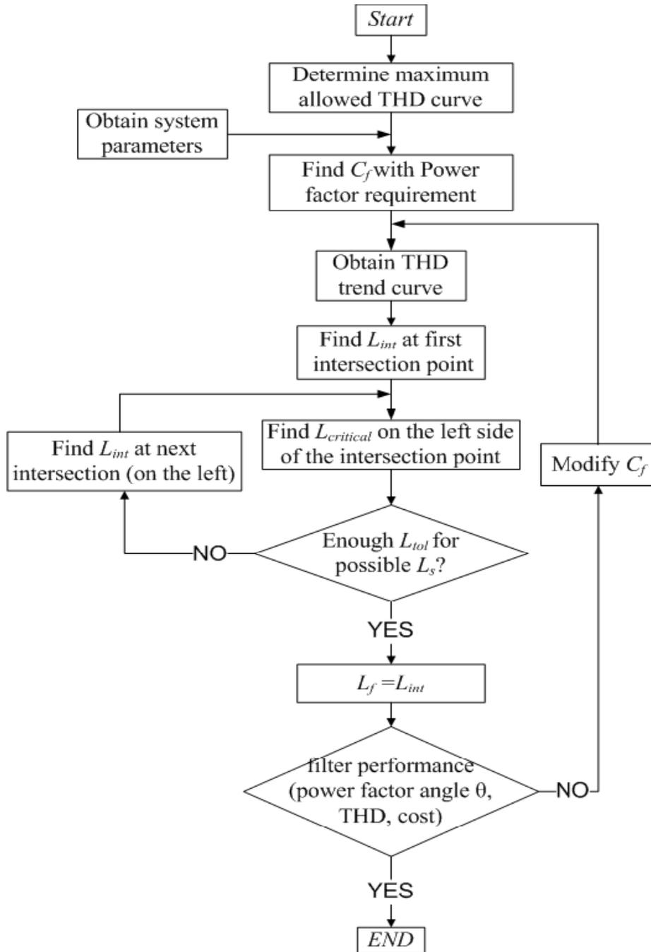
Figure 2.6: Flow chart of filter design procedure
