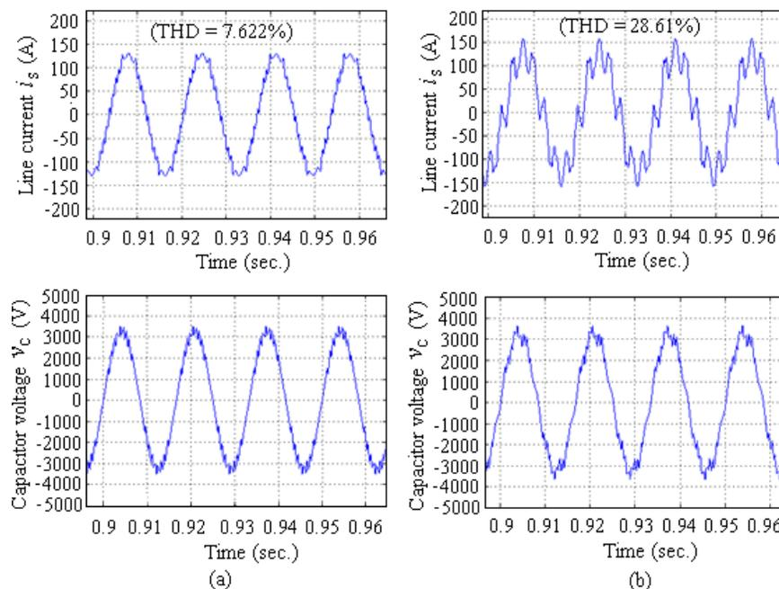
Figure 4.2:  $i_s$  and  $v_c$  of filter design simulation case 2
