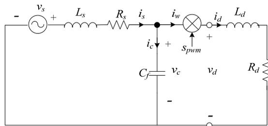
Figure 3.5: Equivalent circuit for DC current ripple analysis
