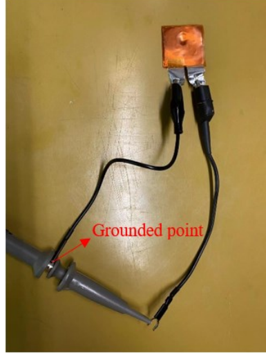
Figure 2.7. An image showing the connection between a sensor and the probe of oscilloscope.
