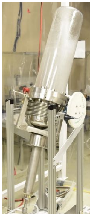
Figure 5.9: Cleaning of the IV with the Revojet spray nozzle.
