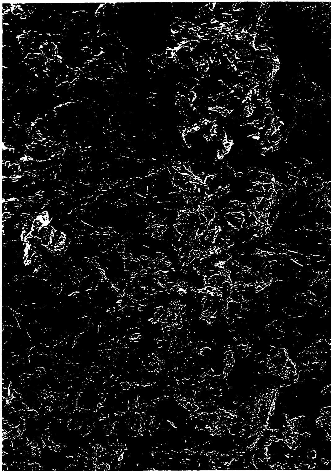
Figure 3.11: Kaolinite clay mixed with deionized water. (Magnification at 500X: — 10 microns)
