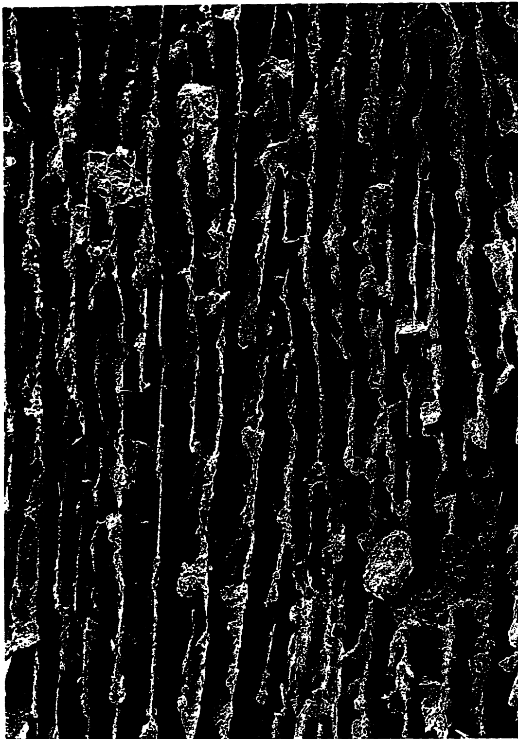
Figure 3.18: Kaolinite clay mixed with MFT pond water and heated to 80 degrees celcius. (Magnification at 500X: — 10 microns)
