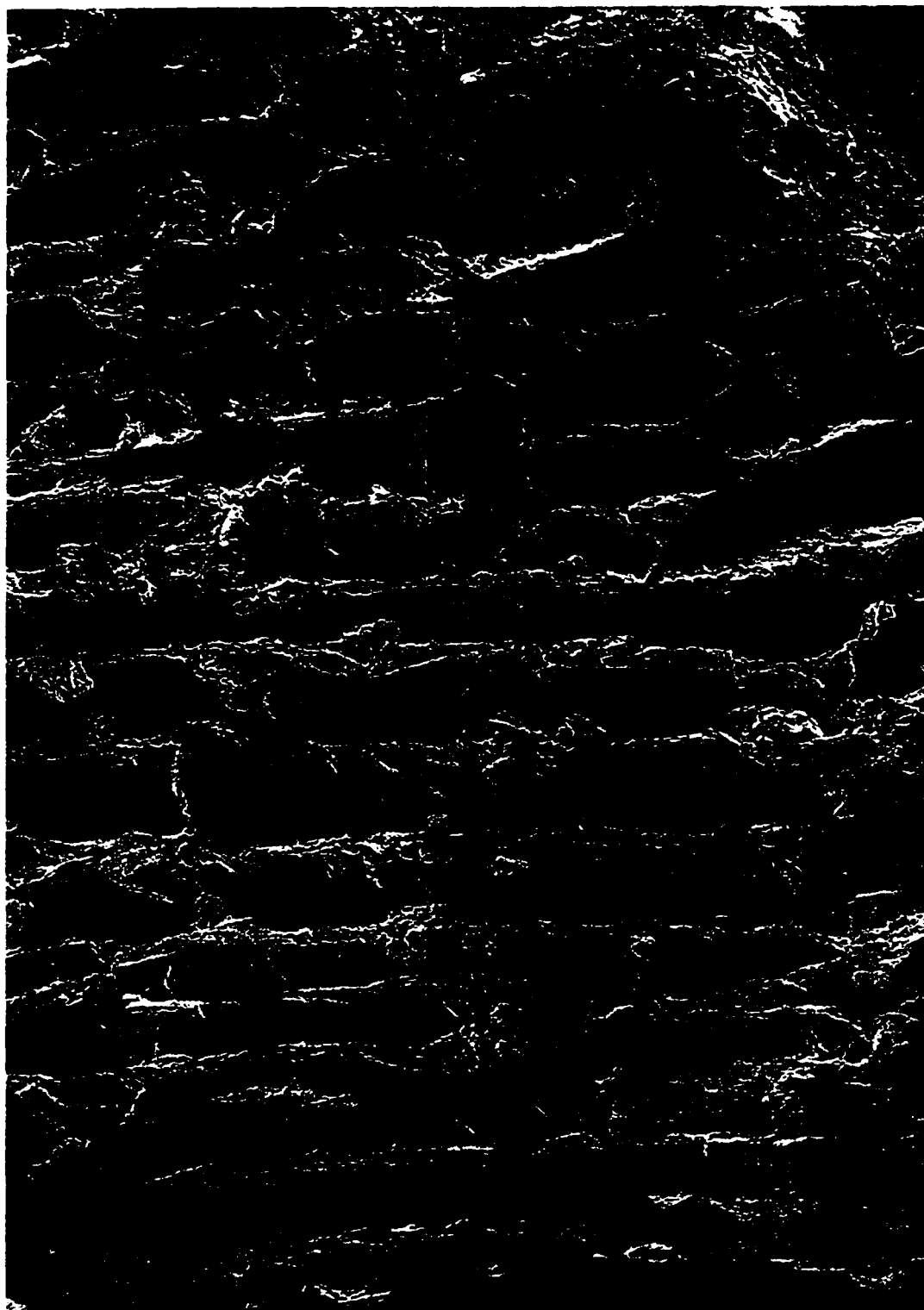
Figure 4.21: CT with 55% clay content MFT mixed with 2500g/m 3 of laboratory grade gypsum. (Magnification at 500X: — 10 microns)
