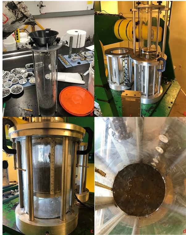
Figure 21 - Dispensing Tailings Material to the Consolidation Cell
