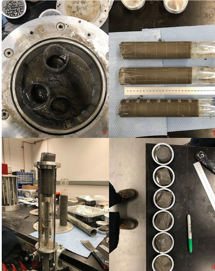
Figure 16 - Push Tube Sampling Technique
