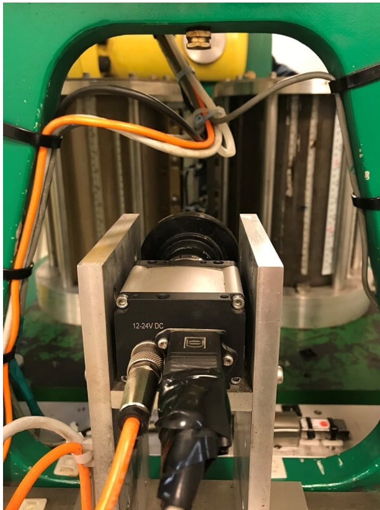
Figure 14 - HD Camera Setup for Interface Settlement Monitoring
