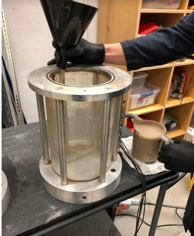
Figure 20 - Funneling Kaolinite Slurry into Consolidation Cell
