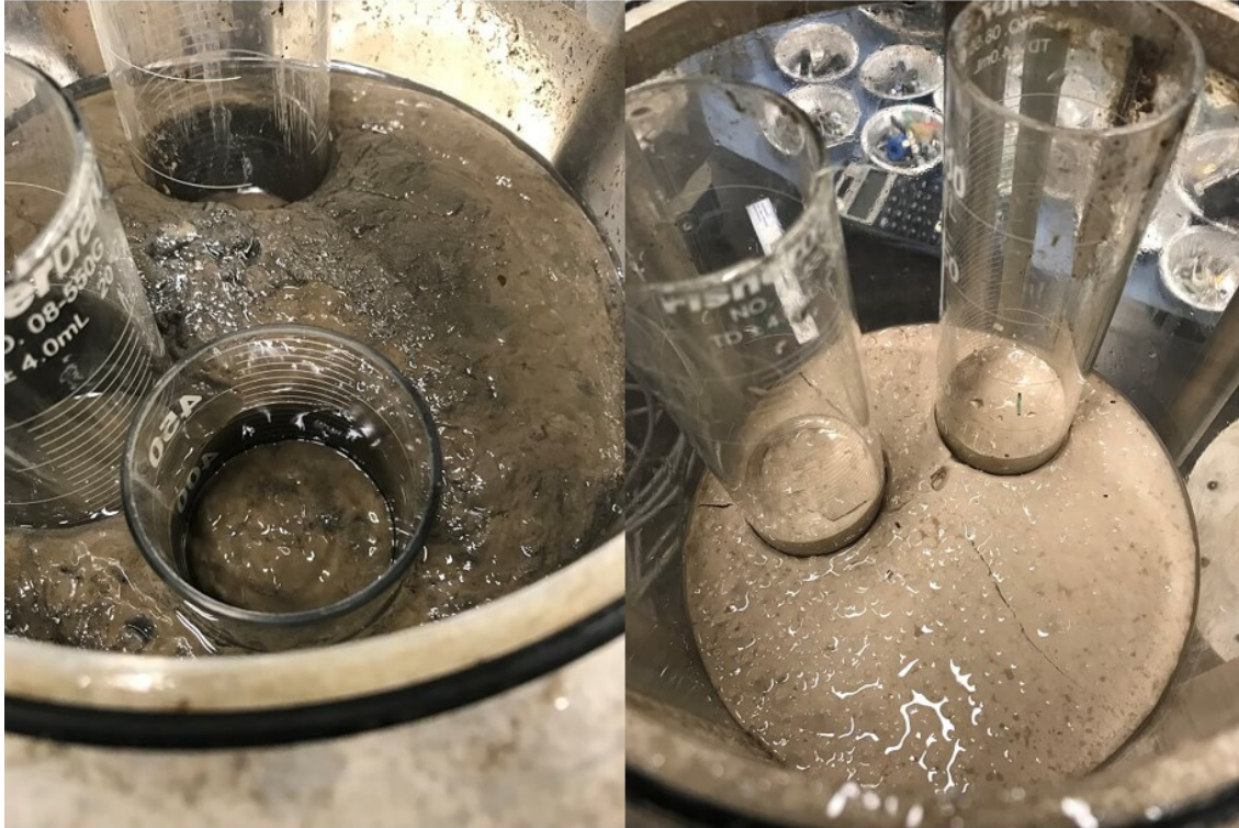
Figure 17 - Push Tube Sampling Technique in Consolidated FFT (Left) and Kaolinite Slurry (Right)
