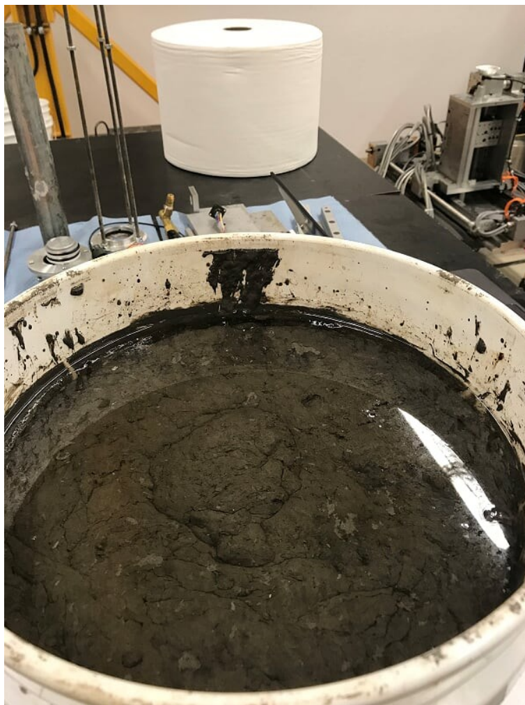
Figure 9 - FFT Mixture After Flocculation
