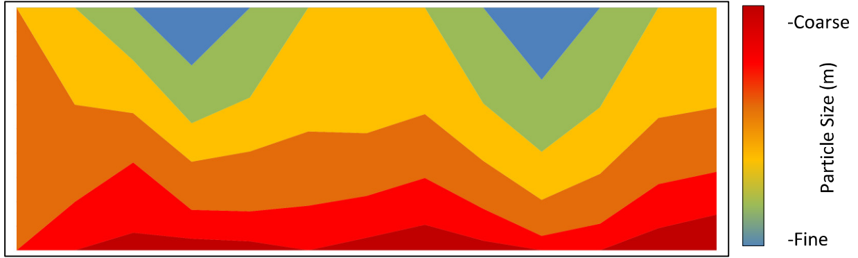
Figure 48 - d_{50} Contours of the Type I North Face (after Chi (2010))
