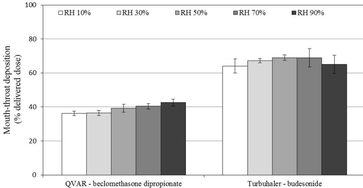
**Figure 4:** Mouth-throat deposition for the QVAR pMDI and Turbuhaler DPI in the Alberta Idealized Child Throat setup at varying RH, expressed as a percentage of delivered dose. Error bars denote standard deviations (n=5).
