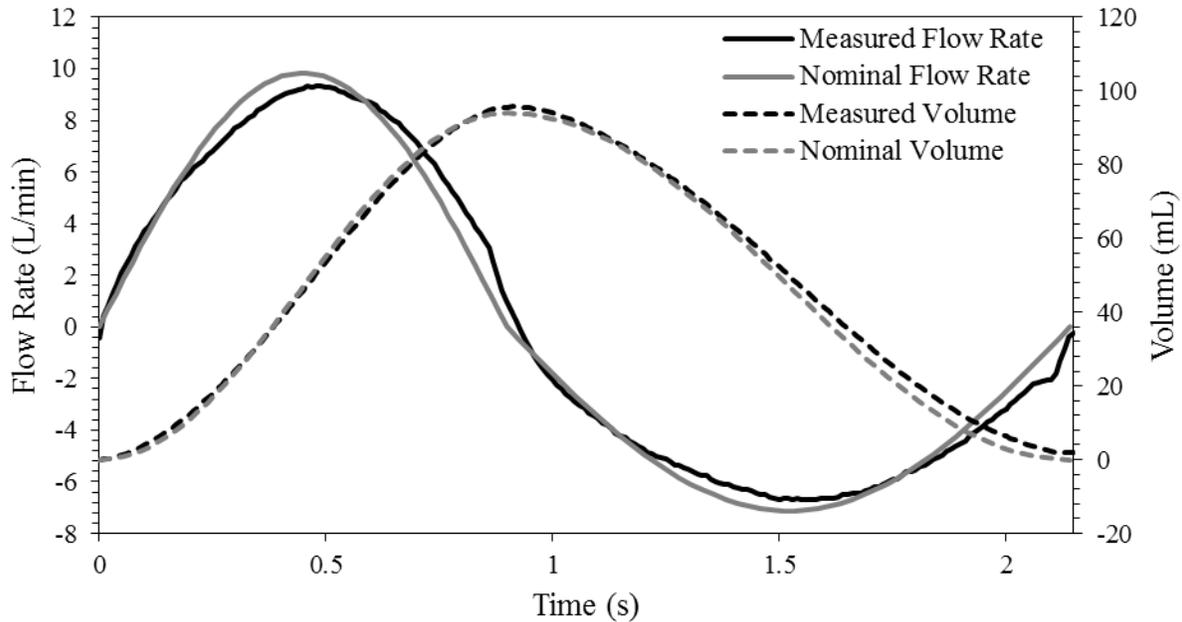
**Figure 8:** Comparison of measured and nominal breathing profiles delivered through the idealized infant geometry using the bias flow experimental setup. Positive flow rate indicates inhalation, negative flow rate indicates exhalation.
