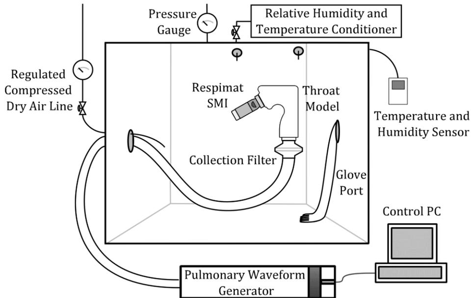
**Figure 15:** Experimental setup used to measure deposition from the Respimat SMI in the Alberta Idealized Child Throat and Bickmann *et al.* idealized throat under controlled environmental conditions.
