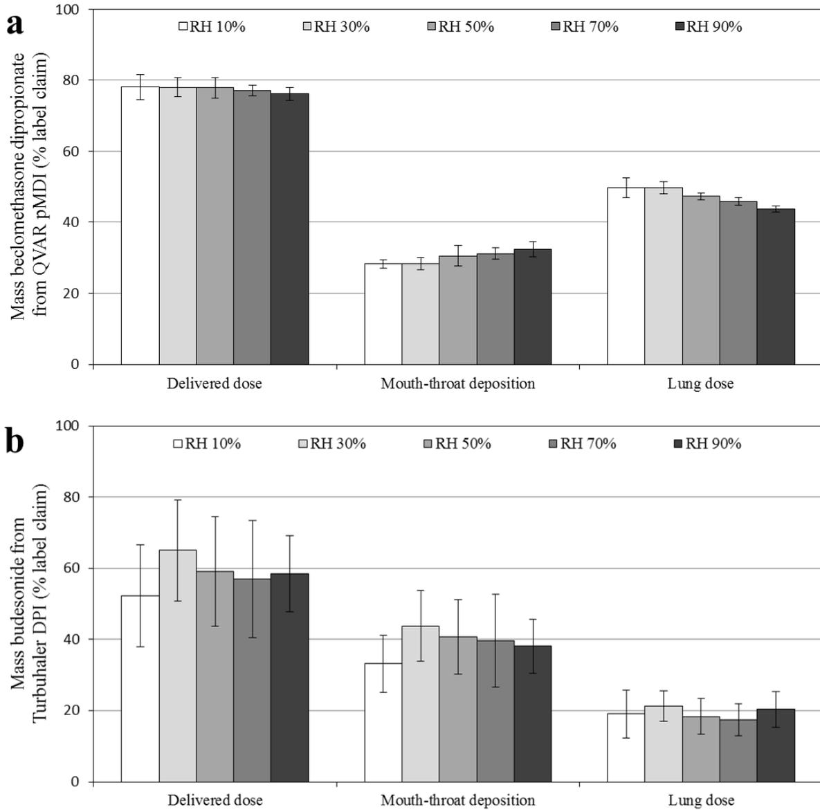
**Figure 3:** Mean deposition of a) the QVAR pMDI and b) the Turbuhaler DPI measured in the Alberta Idealized Child Throat under varying RH. Delivered dose, mouth-throat deposition, and lung dose are expressed as a percentage of the label claim for each device. Error bars denote standard deviation (n=5).
