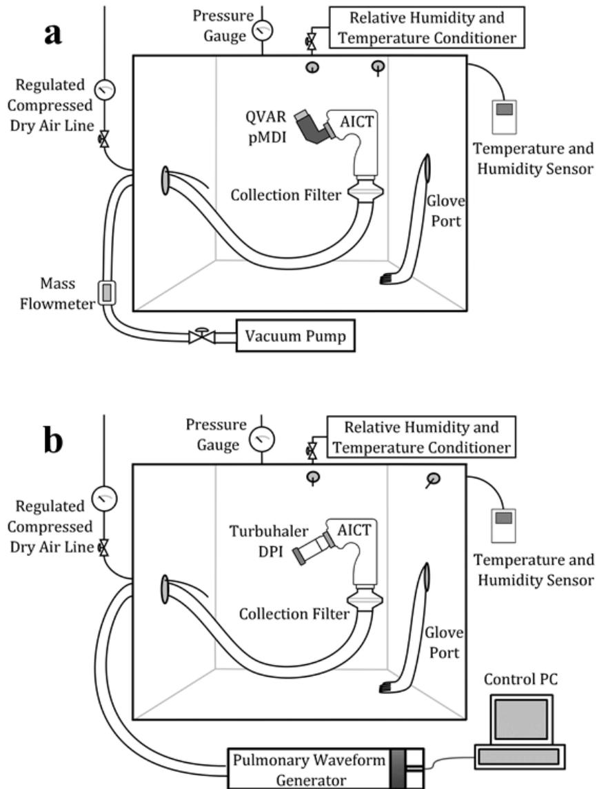
**Figure 2:** Experimental setup for a) QVAR pMDI with a constant flow rate set by a vacuum pump and b) Turbuhaler DPI with a time-variant flow profile supplied by a pulmonary waveform generator. AICT = Alberta Idealized Child Throat.
