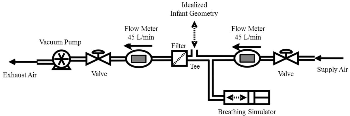
**Figure 7:** Schematic of the bias flow system used to provide simulated breathing patterns to the idealized infant geometry and ensure efficient aerosol collection on the downstream filter.
