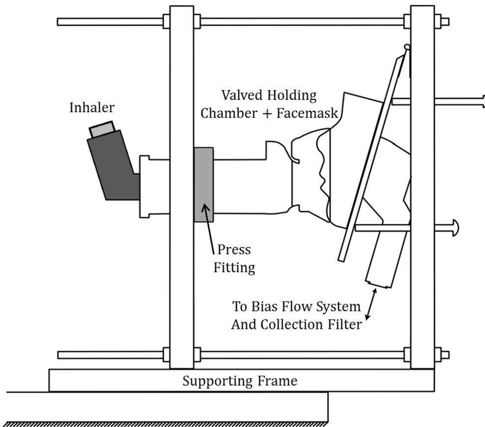
**Figure 6:** Experimental setup used to attach the valved holding chamber plus inhaler to the idealized infant geometry, with the outlet of the geometry leading to the bias flow system and collection filter.
