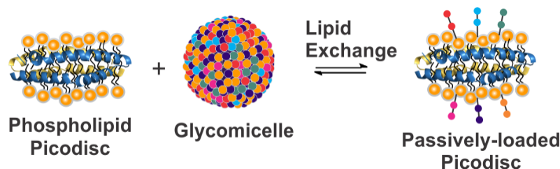
Figure 6.2 The schematic figure of passively-loaded PD formation through lipid transfer between phospholipid PD with GLs in the form of glycomicelle.
