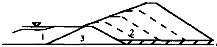
Downstream method of tailings construction
