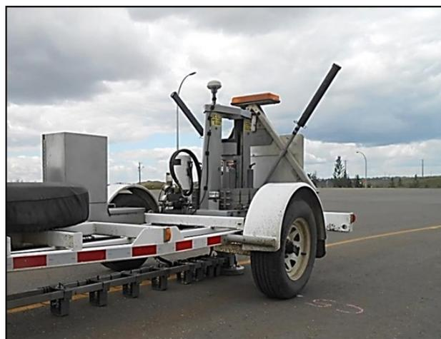
**Figure 2-4 FWD equipment during field testing.**
